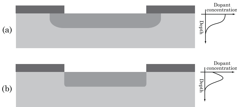
Figure 2.13 Doping profiles after diffusion (a) and ion implantation (b).
