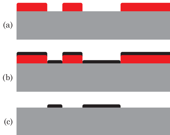
Figure 2.5 Lift-off processing steps: (a) spinning and patterning of the photoresist layer; (b) evaporation of the metal thin film; and (c) removal of the photoresist layer and excess metal.
