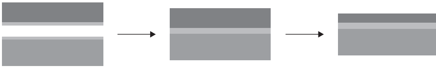
Figure 2.15 Fabrication of SOI wafers through bonding: two oxidised wafers are bonded together and the desired device layer thickness is achieved through thinning the top wafer.
