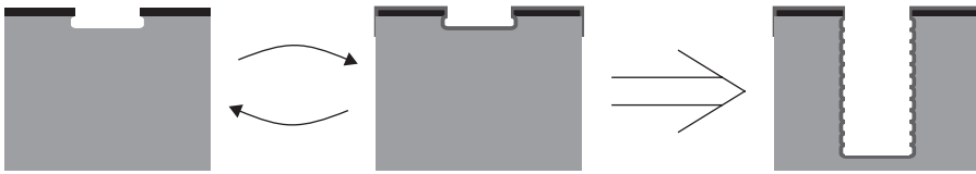
Figure 2.10 Subsequent etch and deposition cycles in a DRIE process and the resulting scallop-like edges on sidewalls.
