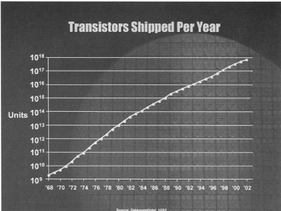
FIGURE 15.6. Plot of the total number of transistors shipped by Intel by year from 1968 to 2002. (Reproduced with kind permission of Intel, http://www.intel.com/research/silicon/mooreslaw.htm ).
