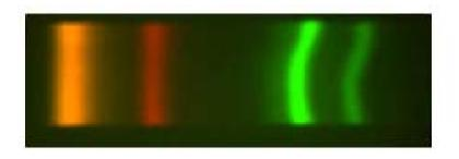
FIGURE 7.21. Isoelectric focusing of proteins PE, APC, and GFP in a 2 cm  $\times 300 \ \mu m \ \times 5 \ \mu m$  PDMS microchannel. Three proteins are completely resolved with band thicknesses below 100  $\mu m$ , and the GFP is subfractionated into two bands. (Courtesy of P. Dutta and C.F. Ivory.)
