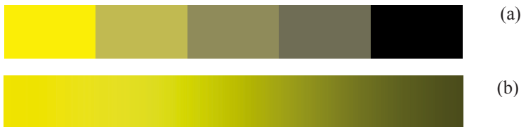
Fig. 4.24 (a) Multilayer model and (b) functional gradient model (using functionally graded elements).
