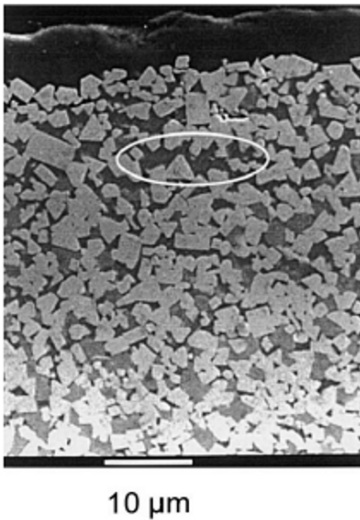
Fig. 3.23 Cobalt enriched zone (example marked) in a graded WC/Co hard metal.
