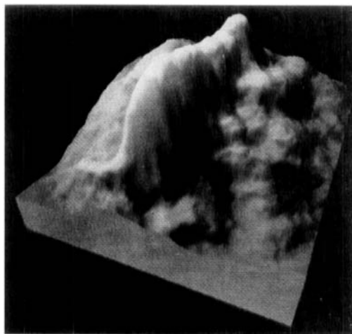
Figure 143. 5 \mu\text{m} \times 5 \mu\text{m} PSTM image of E. coli embedded in buffer salts. The height range is 3 \mu\text{m} , and the image was obtained with He-Ne laser radiation (Reddick et al., 1990).
