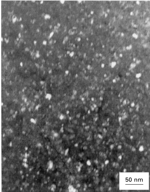
8.2 Si-C-N ceramic synthesized by polymer thermolysis and subsequent crystallization for 240 h at 1400 °C in a compression creep experiment, consisting of Si 3 N 4 and SiC crystallites and turbostratic C in a residual amorphous matrix. Dark field TEM image courtesy of A. Bauer.
