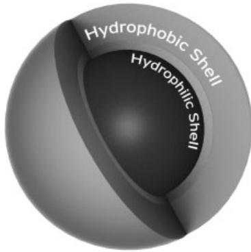
Figure 1.12. Diagram of PEBBLE nanosensor [79]. Reproduced with permission from Analytical Chemistry, Vol. 76, Y.-E. L. Koo et al., Copyright (2004) American Chemical Society. Real-time measurements of dissolved oxygen inside living cells by organically modified silicate fluorescent nanosensors, p. 2498–2505.
