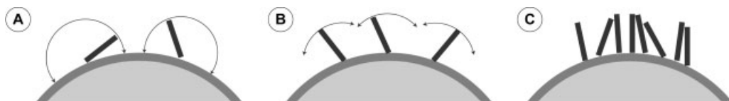
Fig. 6.5. Formation of oligonucleotide layers on gold nanoparticle surfaces. The conformation depends on the DNA molecule density on the surface. (A) At very low surface coverage, no steric interactions occur between strands on the surface. (B) For higher molecule densities, collisions will occur between the ends of neighboring oligonucleotides, restricting the possible strand orientations and forcing the DNA strands to “stand up”. (C) As surface coverage increases, the oligonucleotides approach their theoretical limit of a densely packed monolayer of “standing up” DNA strands. (Modified after Ref. [92].)
