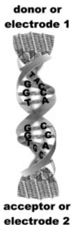
Figure 5.2. (a) Diagram of the DNA double-stranded helical structure. (b) Possible interconnection of DNA fragment with two electrodes or an acceptor and a donor group for transport studies.
