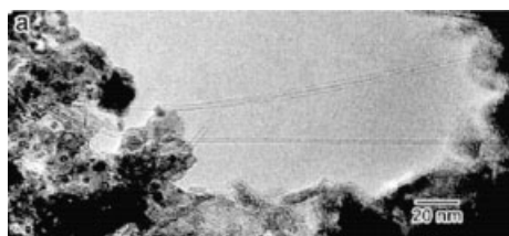
Fig. 1.3. Transmission electron microscopy (TEM) image of an SWNT synthesized by chemical vapor deposition (CVD). (Reprinted with permission from Ref. [37], © 2001, The American Chemical Society).
