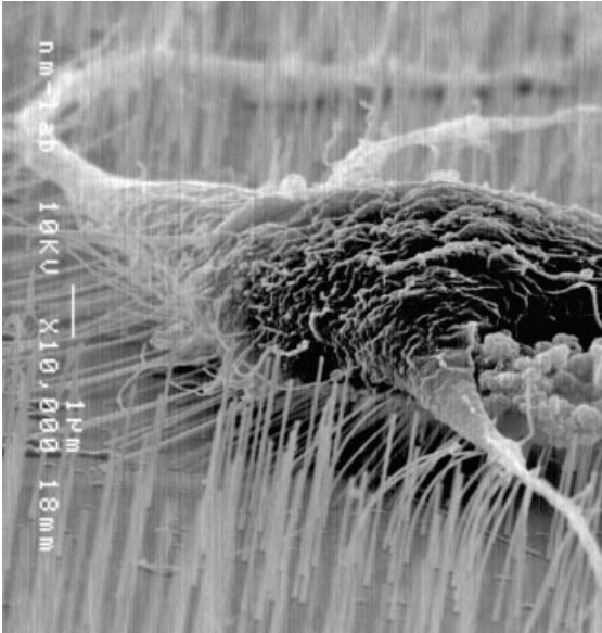
Figure 12.22. Neurons supported on a surface consisting of randomly located epitaxial GaP nanowires on GaP substrate, revealing a healthy appearance. Note that some wires are bent and in some cases wires are inserted into the neuronal cells and processes. (From Ref. [149].)
