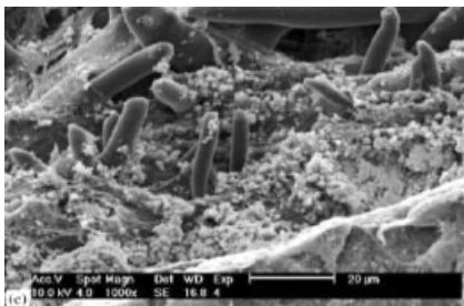
Fig. 1.40. SEM showing a cell nanofiber construct after 4 weeks in culture. Globular accretions, abundant calcification and collagen bundles can be seen. (Adapted from Ref. [178] with permission from Elsevier.)
