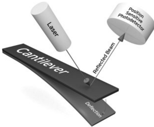
Figure 1.29. Typical optical measurement of cantilever deflection [130]. Reproduced with permission from Nickolay V. Lavrik, Review of Scientific Instruments , 75, 2229 (2004). Copyright 2004, American Institute of Physics.
