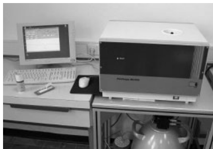
Fig. 7.1. Benchtop 9 GHz ESR-spectrometer (X-band) with temperature unit (below the spectrometer).
