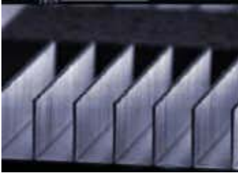
Fig. 7.14 ICP-depth etching with high aspect relation in crystalline silicon
