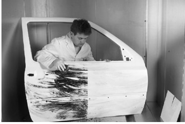
Fig. 5.17 Partial coverage of a car door with a layer of nanoparticles for dirt rejection
