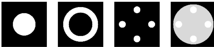
Fig. 7.17 Off-axis exposure for the reduction of diffraction effects, from left to the right: Standard, annular, quadrupole CQUEST I, quadrupole CQUEST II
