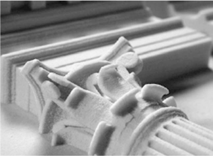
FIGURE 3.3 Example of a complex three-dimensional geometry fabricated using a mass change process — inkjet printing, an additive manufacturing process. (From Digital Design Fabrication Group, MIT Department of Architecture, http://ddf.mit.edu . With permission.)
