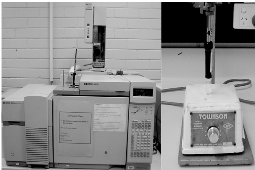
FIGURE 3.9. Typical system of GC/MS with SPME.
