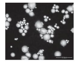
Figure 5.3: Scanning electron micrograph of Co-Cr particles retrieved from tissues adjacent to a human implant at revision surgery. The scale bar at the lower right is 10  $\mu$ m long. Courtesy of Prof. Peter Revell.
