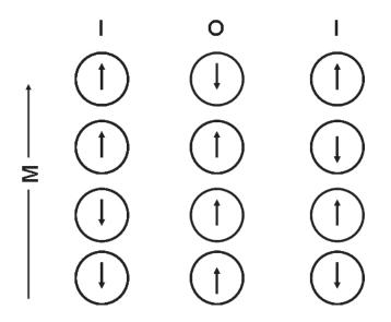
Figure 9.1: A spintronic NAND gate. The two inputs are the left and right columns, and the output is the central column. The physical entities are quantum dots. The upspin state parallel to the global magnetic field **M** represents 1 and the downspin state represents 0. Exchange interaction causes nearest neighbours to prefer antiparallel spins, but if there is a conflict, the global magnetic field biases the output to 1.
