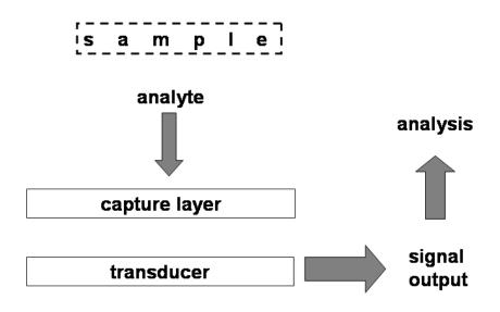
Figure 9.2: A prototypical biosensor. The capture layer concentrates the analyte in the vicinity of the transducer, which reports the concentration of analyte in the capture layer, which is directly related to the concentration in the sample.
