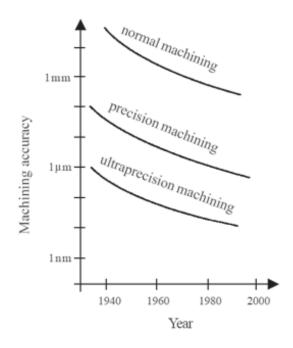
Figure 1.1: The evolution of machining accuracy (after Norio Taniguchi).
