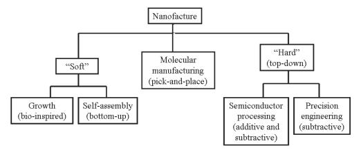
Figure 7.1: Different modes of nanomanufacture (nanofacture) (see text).
