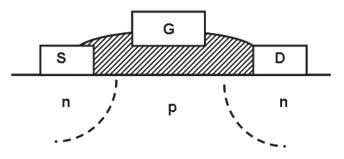
Figure 6.3: A field-effect transistor (FET). Regions marked "n" and "p" are n-type and p-type semiconductors (e.g., appropriately doped silicon). The hatched region is an insulator (e.g., silica). Conductors S, G and D are, respectively, the source, gate and drain. Application of a voltage to G (which plays the role of the coil in the relay) increases the concentration of conduction electrons in the p region and allows current to flow from S to D.
