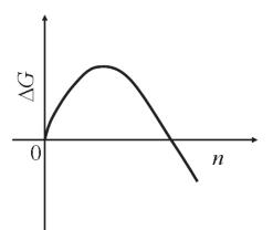
Figure 5.1: Sketch of the variation of free energy of a cluster containing n atoms. The maximum corresponds to the critical nucleus size. Clusters that have managed through fluctuations to climb up the free energy slope to reach the critical nucleus size have an equal probability to shrink back and vanish, or to grow up to microscopic size.
