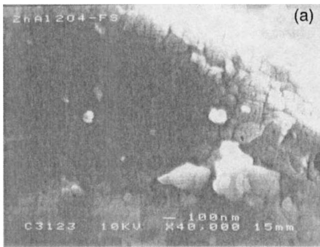
Fig. 7. SEM images of a \text{ZnAl}_2\text{O}_4 pellet (sintered at 1000^\circ\text{C} ): (a) surface morphology and (b) fracture surface.
