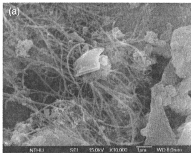
Fig. 6. Morphology on the interlaminar fracture surface of specimen 4S5C5K, diameter of the fibers are <math><100\text{ nm}</math>.
