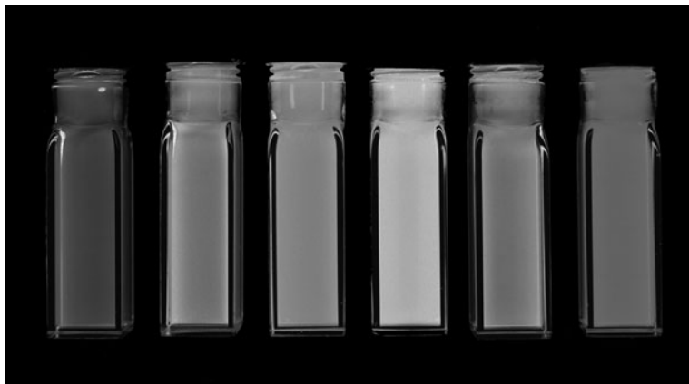
Fig. 4.3 Vials of cadmium selenide nanocrystals of various sizes between 3 and 5 nm in diameter, irradiated by ultraviolet light, showing the effect of size on the fluorescence colour of the particles. Image courtesy of Felice Frankel, originally in colour as seen on the back cover of this book. Reprinted with permission from B. O. Dabbousi, J. Rodriguez-Viejo, F. V. Mikulec, J. R. Heine, H. Mattoussi, R. Ober, K. F. Jensen, and M. G. Bawendi. ( CdSe ) ZnS Core-Shell Quantum Dots: Synthesis and Characterization of a Size Series of Highly Luminescent Nanocrystallites Journal of Physical Chemistry B 101 (1997) 9463–75. Copyright 1997 American Chemical Society.
