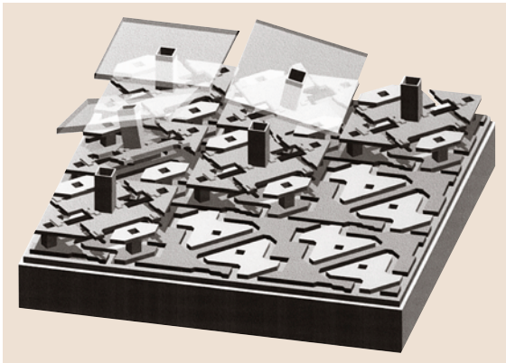
Fig. 36.4 DMD pixel array with tilted and non-tilted mirrors. (Courtesy of Digital Light Processing™, Texas Instruments, Inc.)
