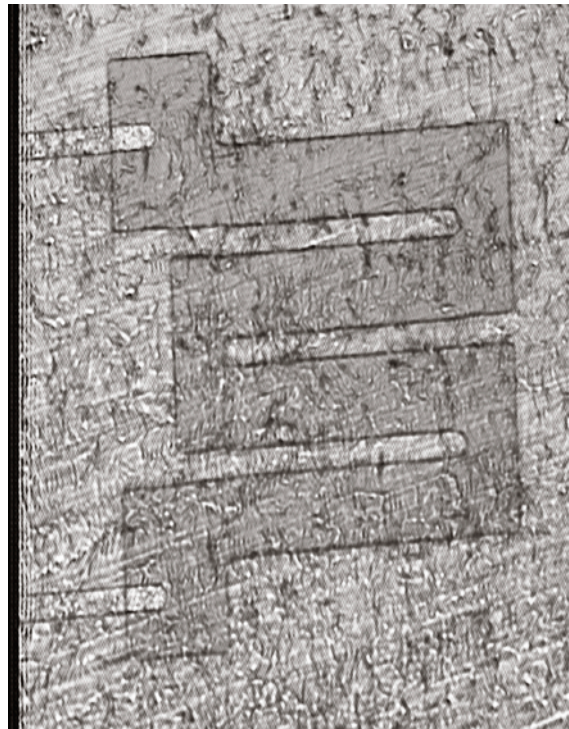
Fig. 32.17 Piezoresistive strain sensor on steel substrate
