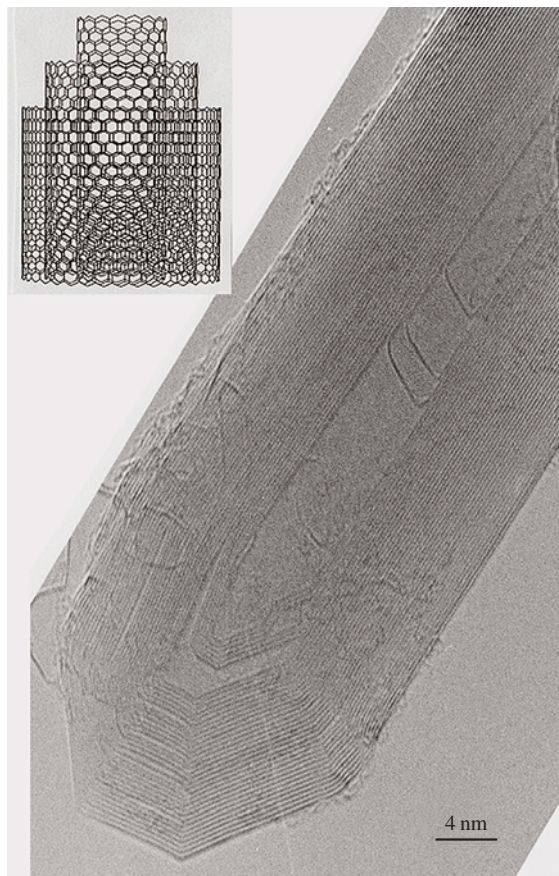
Fig. 3.5 High resolution transmission electron microscopy image (longitudinal view) of a concentric multiwall carbon nanotube (c-MWNT) prepared by electric arc. In insert , sketch of the Russian-doll-like display of graphenes
