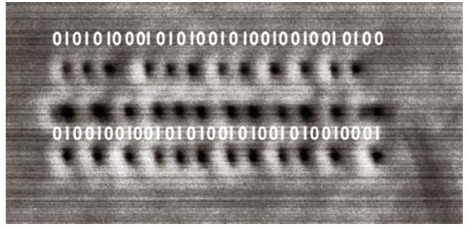
Fig. 31.27 Experimental result of overwriting a bit sequence
