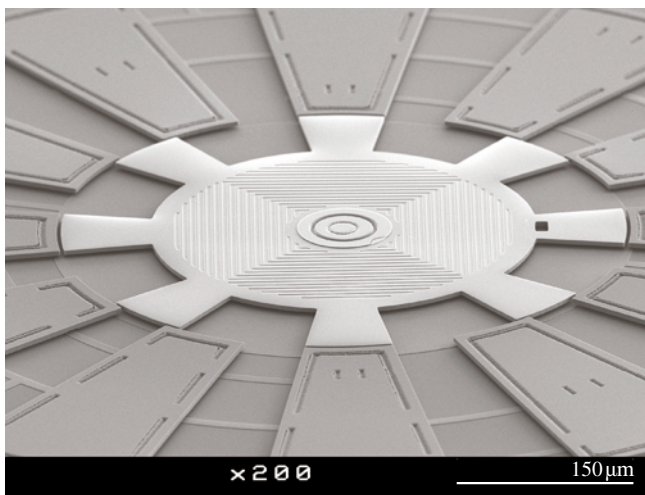
Fig. 7.2 SEM micrograph of a surface-micromachined polysilicon micromotor fabricated using a \text{SiO}_2 sacrificial layer
