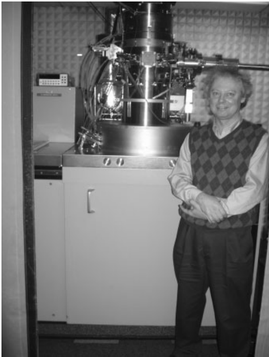
Figure 21 Steven Pennycook, of Oak Ridge National Laboratory, with record setting electron microscope, which took the resolution down to 0.6 Angstrom, less than the diameter of a hydrogen atom. Photo by author.
