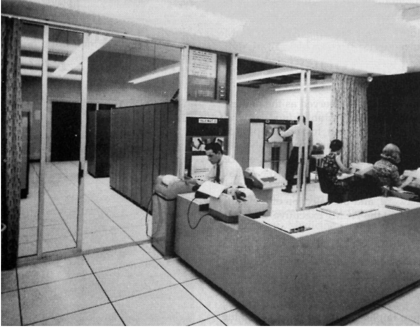
Figure 6.1 DEC PDP-1 computer at BB&N headquarters in Cambridge, Massachusetts. The Massachusetts General Hospital, Hospital Computer Project, Status Report, Memorandum Nine (1966c), p. 9.
