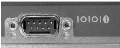
FIGURE 235. Serial port (note “10101” symbol indicating a stream of bits)
