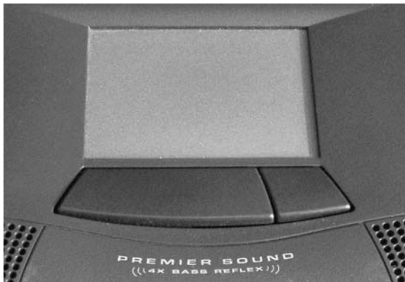
FIGURE T.3 Trackpads are pointing devices that take the place of a mouse on many portable computers.
