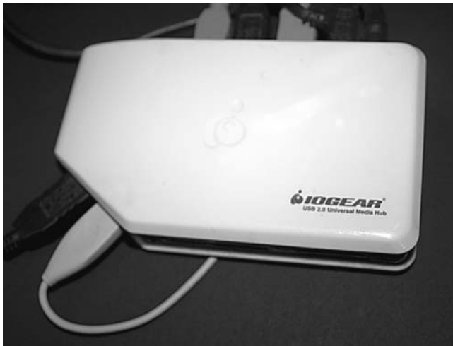
FIGURE H.2 A typical USB hub.
