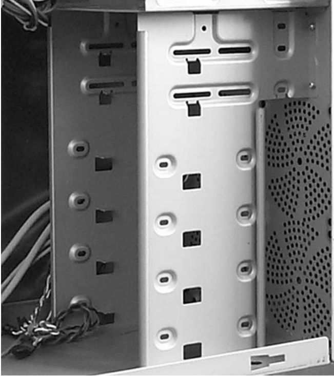
FIGURE B.4 This computer enclosure supports up to six internal drives as well as four external ones.
