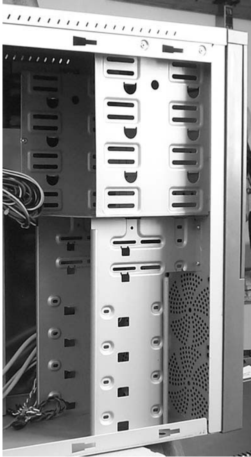
FIGURE C.6 The chassis of your enclosure is the skeleton that provides structural support.
