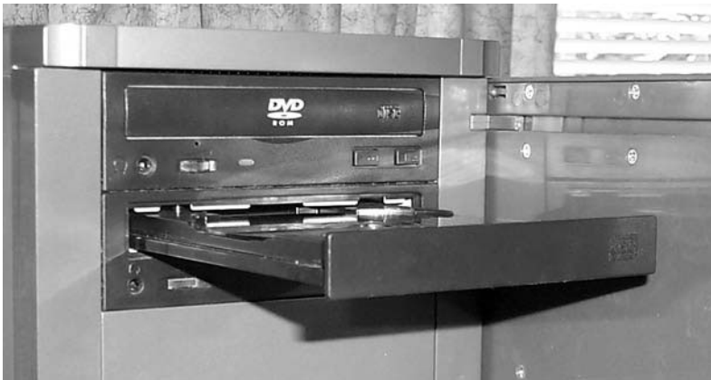
FIGURE B.6 The bezel on this CDR covers the internal mechanisms and provides support for the eject key and a status light.
