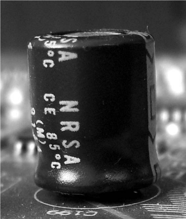
FIGURE C.3 A capacitor is a device much like a storage battery that holds an electrical charge until such time as the circuit on which it is installed requires the energy.
