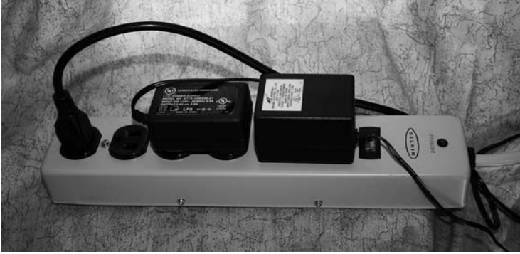
FIGURE A.3 Many devices used alongside the computer require AC adapters to provide their current.
