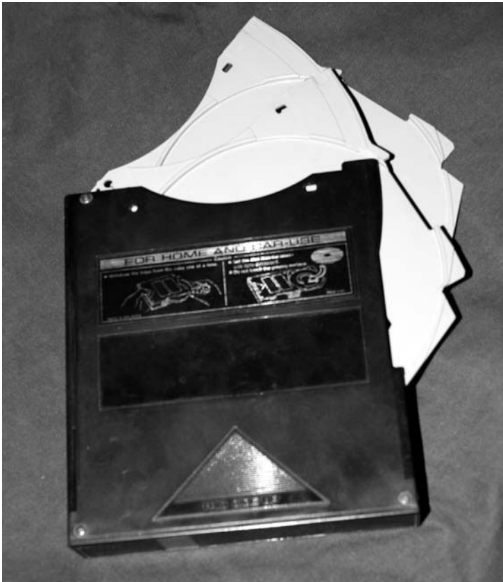
FIGURE C.2 This six-disk caddy is used in an audio CD player.
