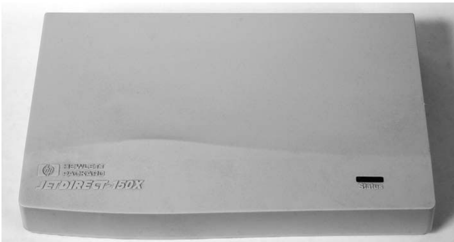
FIGURE T.4 This HP Jetdirect is an example of a stand-alone transceiver.
