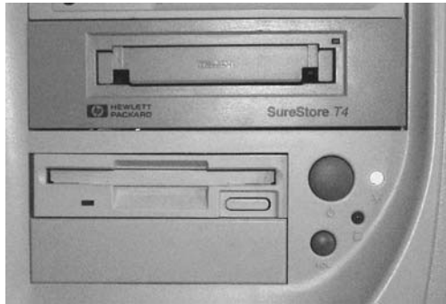
FIGURE A.5 The drives on the front of this computer enclosure feature activity lights to indicate when the drives are busy.
