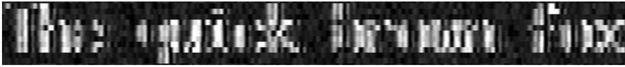
Fig. 1. The top image shows a short test text displayed on a CRT monitor. In the bottom image, the compromising emanation from this text was picked up with the help of an AM radio receiver (tuned at 450 MHz, 50 MHz bandwidth) and a broadband UHF antenna. The output was then digitized, averaged over 256 frames to reduce noise, and finally presented as a reconstructed pixel raster
