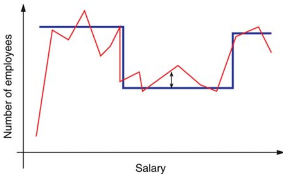
Histograms on Streams. Figure 1. A histogram of three buckets for a frequency vector of data (jagged polygon). Often the goal is to minimize the sum of square between the data vector and histogram by choosing the bucket boundaries and heights for the histogram.
