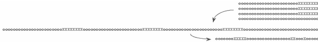
Figure 5. Row-major linearization of a 2-D cell array, followed by compression; “X” cells show some region getting scattered on disk, thereby rendering all but horizontal access inefficient
