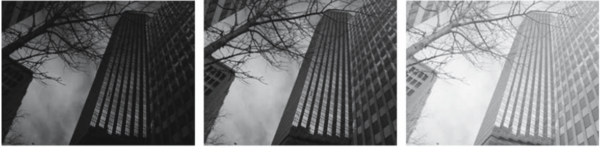
Exposure Values. Figure 1. Examples of images acquired using different exposure settings: (left) low-exposure, (middle) medium exposure, and (right) high-exposure.
