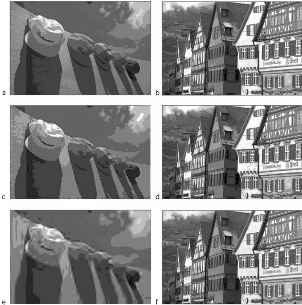
Advances in Image and Video Quality Assessment. Figure 1. (a) Original “Caps” image (b) Original “Buildings” image (c) JPEG compressed image, MSE = 160 (d) JPEG compressed image, MSE = 165 (e) JPEG 2000 compressed image, MSE = 155 (f) AWGN corrupted image, MSE = 160.
