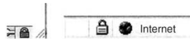
Online Multimedia E-Commerce. Figure 1. Web Browsers Netscape (left) and Internet Explorer (right) indicating SSL.
