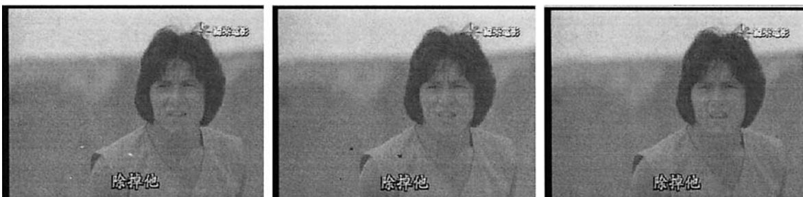
Digital Inpainting. Figure 5. Video inpainting results – the damaged frame (left), the detected spikes shown in red (middle), and the repaired frame (right).
