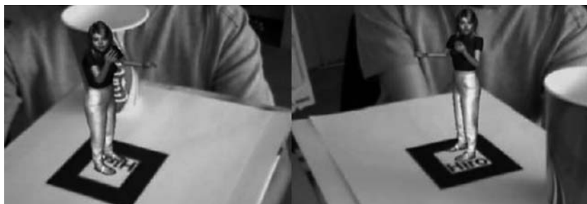
Interactive Virtual Humans in Mobile Augmented Reality. Figure 5. Self-adaptive animation based on AR user perspective.
