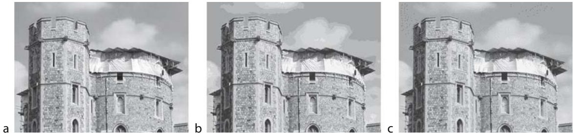
Color-Mapped Imaging. Figure 5. Dithering in color-mapped imaging: (a) true color image with 26,124 colors, (b) indexed image with 16 colors obtained without using advanced color reduction techniques, (c) masking the band artifacts using a dithering technique in [15].
