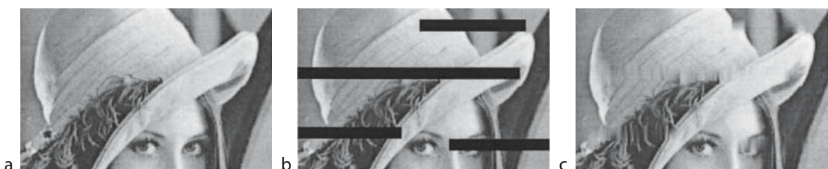
Image Inpainting. Figure 1. Image inpainting: (a) original image, (b) damaged image with missing rows ( blocks ) due to wireless transmission, (c) reconstructed image by an inpainting technique.
