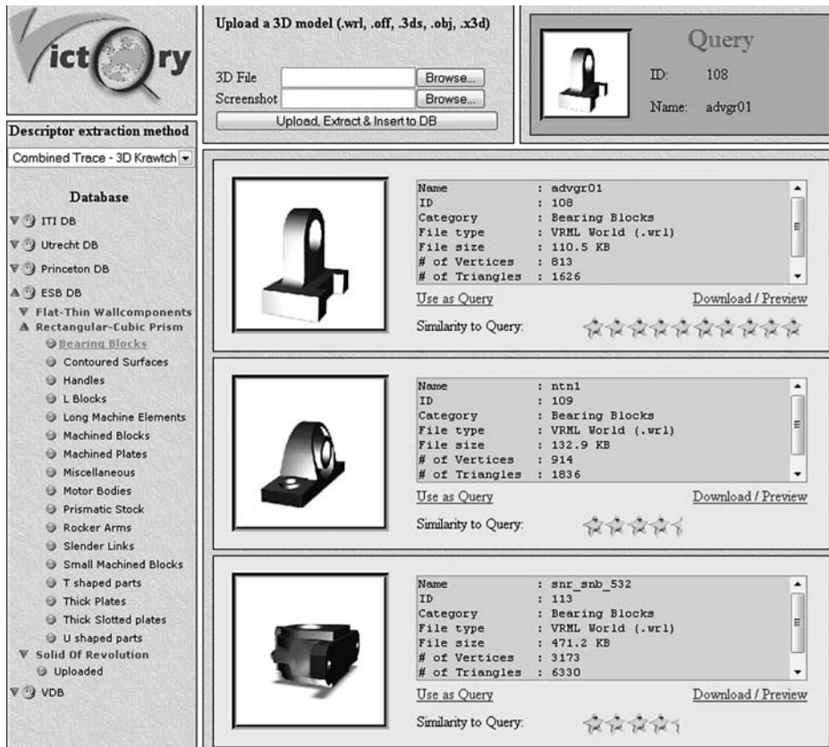
Three Dimensional Content-Based Search and Retrieval of CAD Objects. Figure 3. Search and retrieval of CAD objects ( http://www.victory-eu.org/ ).
