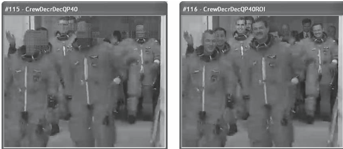
Privacy and Video Surveillance. Figure 3. Decoded and decrypted frame under extreme compression (left), and the same decoded and decrypted frame with a fixed ROI high quality (right).
