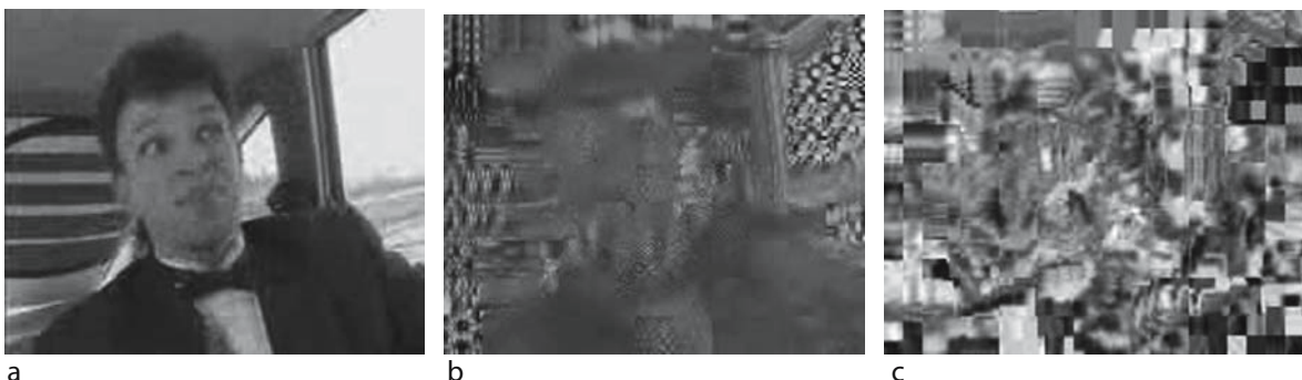
End-to-End Security for Multimedia Adaptation. Figure 3. Scrambled predicted coded frames using the joint encryption/compression techniques. (a) Unscrambled frame, (b) Scrambled frame using [0], (c) Scrambled frame using [0].
