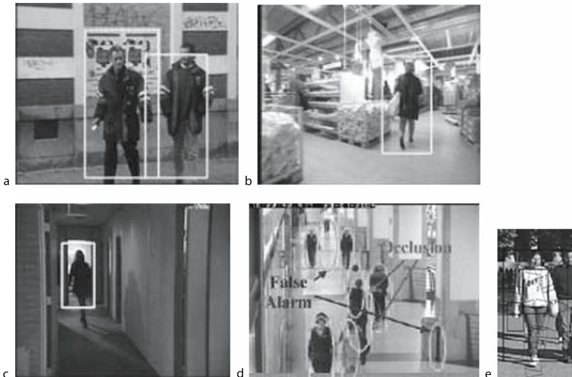
Person Detection in Images and Video. Figure 4. Illustration of the results provided by the person detection approaches. (a) Detection of more than one persons in the same image, (b & c) human detection under difficult monitoring conditions (aliasing in (b) and illumination problems & shadowing in (c)), (d) results provided by the Hydra system [19], (e) part-based person detection [18].
