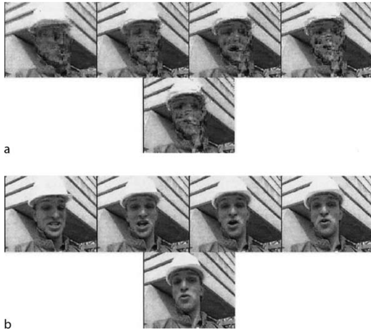
Video over IP. Figure 2. Sample visual results of video delivery quality using (a) best-effort and (b) QoS.
