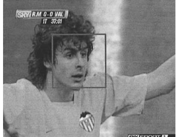
Video Automatic Annotation. Figure 3. Face detection using the Viola and Jones algorithm.
