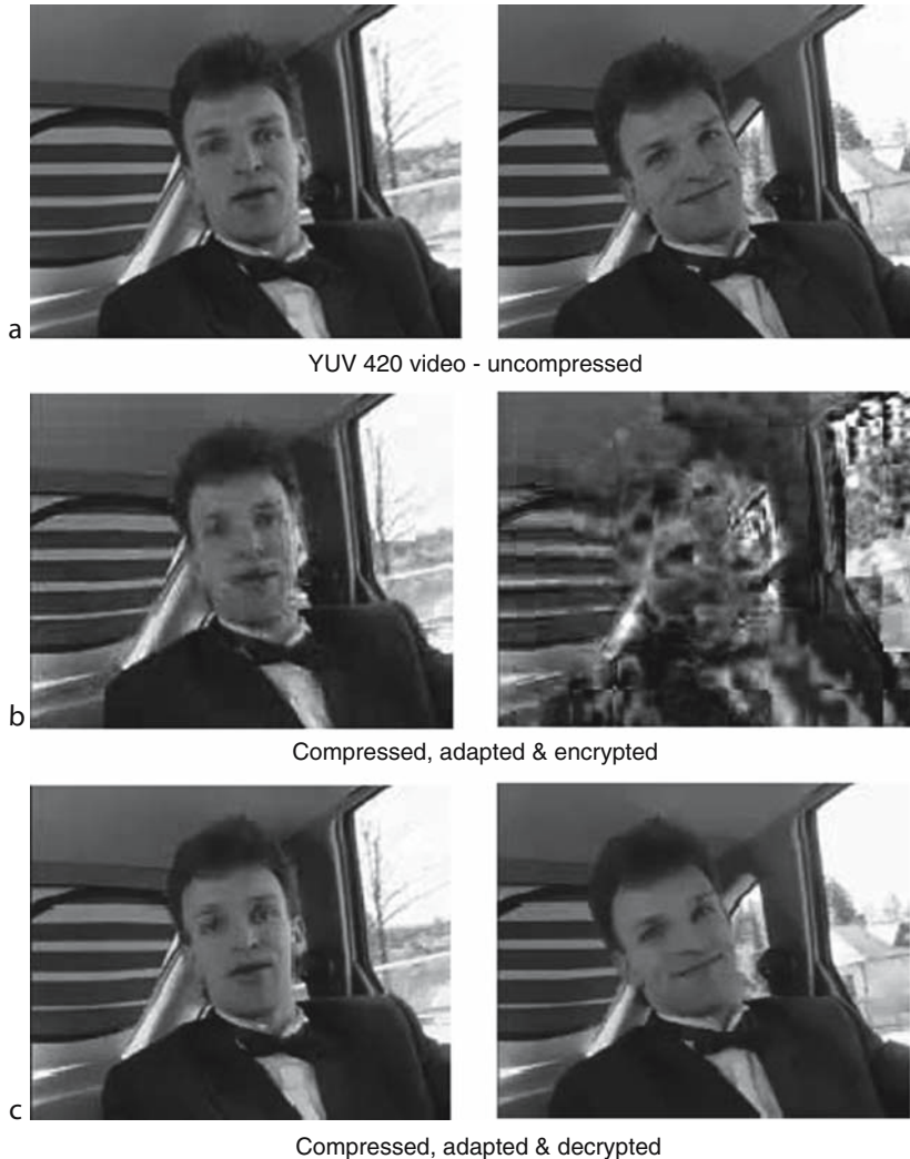
MPEG-21 Based Video Adaptation with Encryption and Authentication. Figure 9. Sample video output (Carphone) (a). YUV 420 video – Uncompressed (b). Compressed, adapted and encrypted. (c). Compressed, adapted and decrypted.
