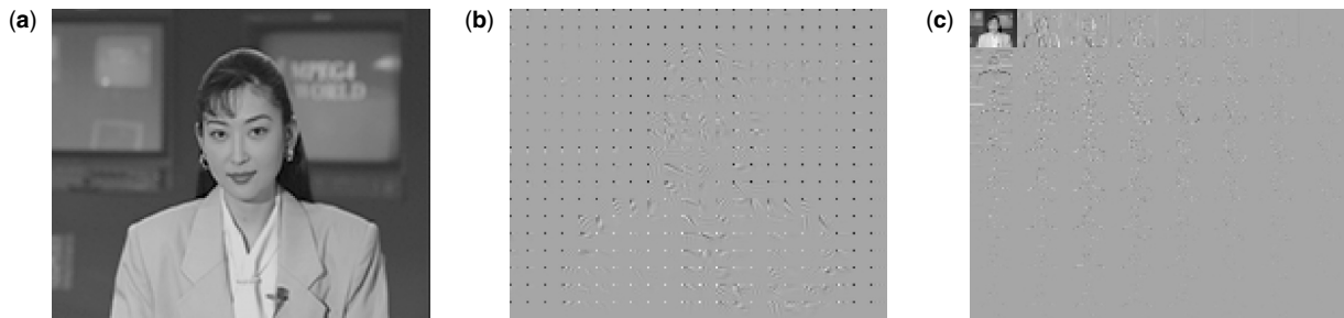
Figure 4. Example of a blockwise 2D DCT of an image: (a) original image (144 × 176 pixels); (b) transformed image (blocksize 8 × 8, 18 × 26 blocks); (c) transformed image after reordering of coefficients (8 × 8 subimages of size 18 × 26).
