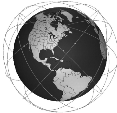
Figure 3. Orbital geometry for the Globalstar constellation, an example of a rosette constellation (from Thurman and Worfolk [8], used with permission).
