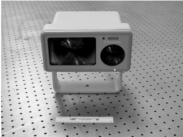
Figure 2. Photo of 0.85- \mu\text{m} noncoherent LED-based FSO system from PlainTree used for short/moderate indoor applications. Photo is that of a PlainTree Model 340 system.
