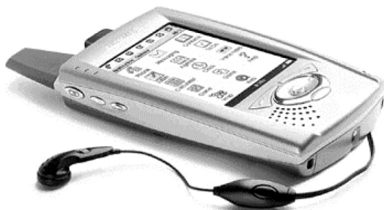
Figure 7. Next-generation PDA device with pen and speech based input, integral GPS and GPRS connectivity [9].
