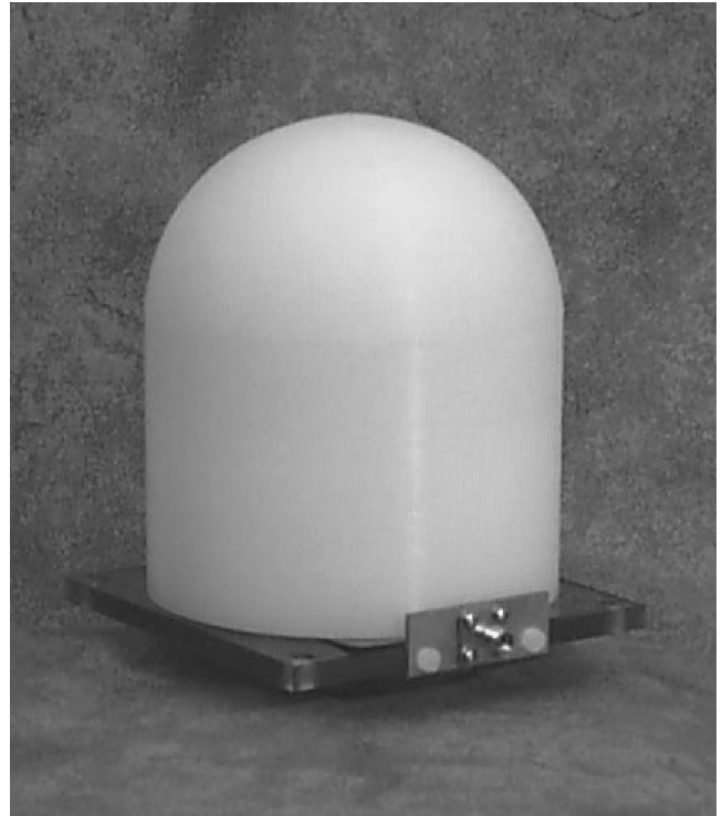
Figure 16. Photograph of millimeter wave lens-coupled proximity-coupled microstrip patch antenna.
