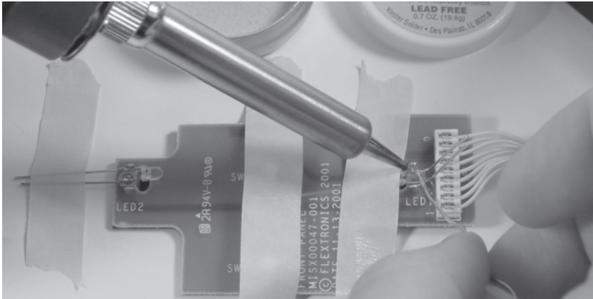
Figure 3-10: Soldering the LEDs in place. Note how the board and the LEDs are taped in place using masking tape.
