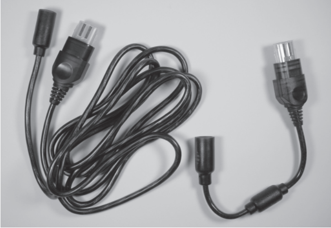
Figure 4-1: (Left) an Xbox game controller extension cable. (Right) an Xbox breakaway cable.
