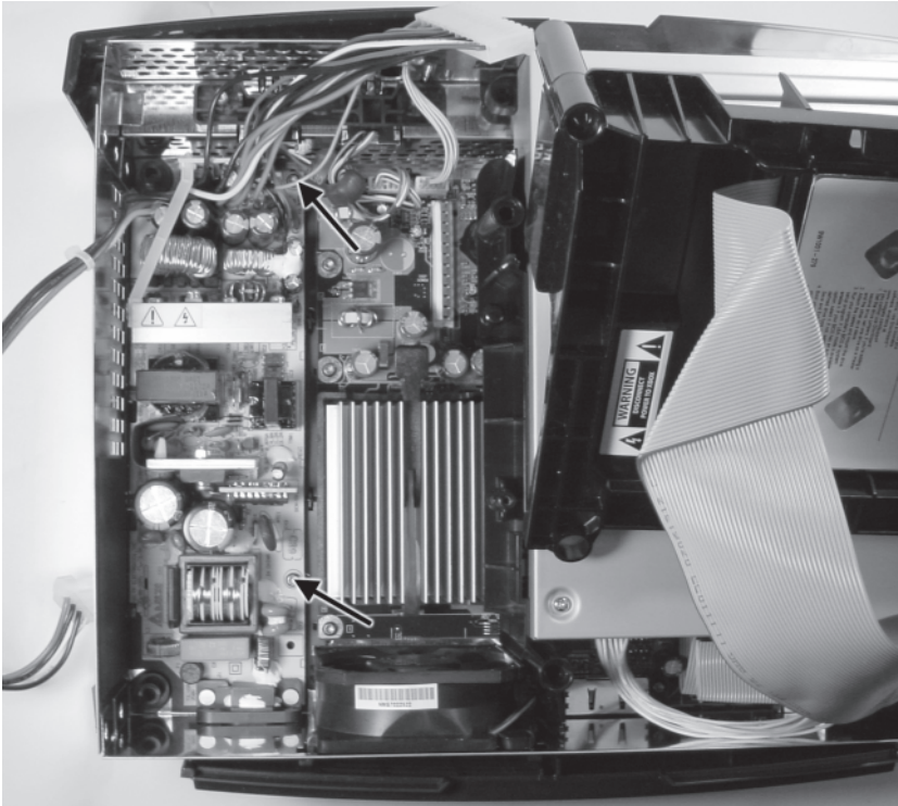
Figure 5-7: Location of the two power supply mounting screws.
