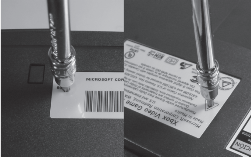
Figure 1-4: Location of the screws hidden by the serial number and product certifications labels.
