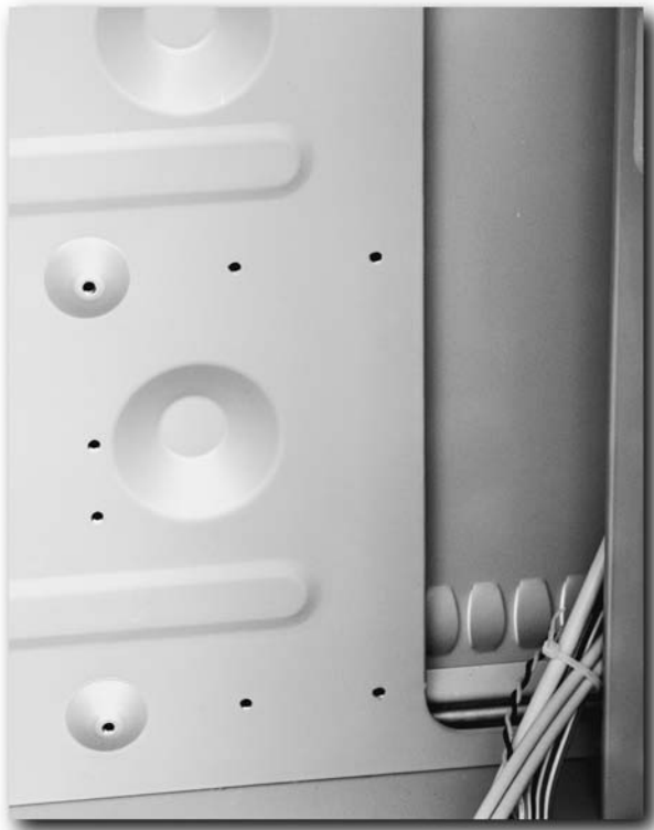
FIGURE 14-3: Lots of motherboard mounting points in a single case!
