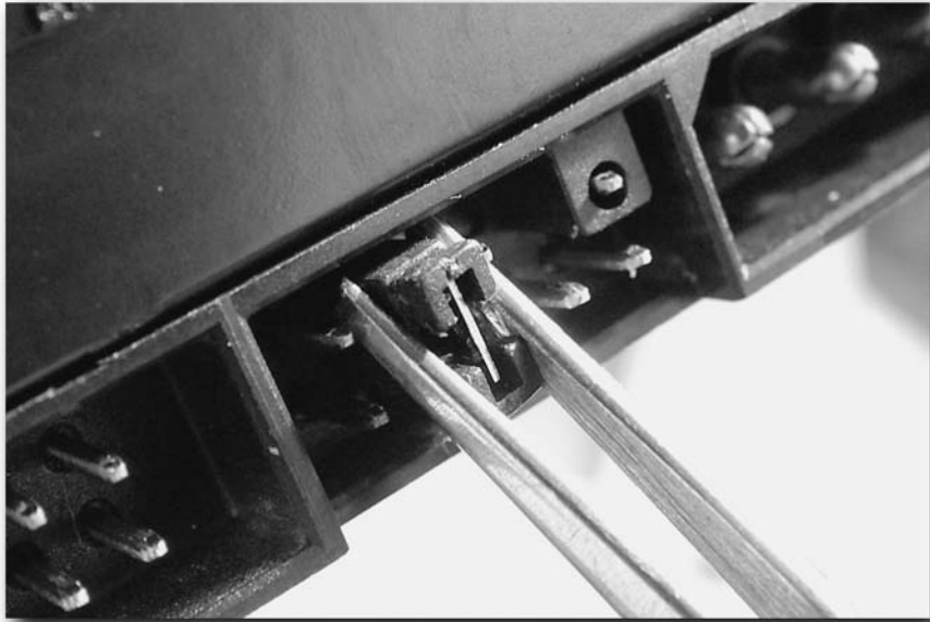
FIGURE 15-8: Configuring the jumpers for cable select.
