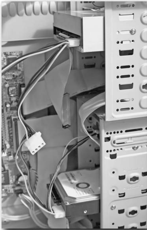
FIGURE 15-15: Optical drive complete with power and data cable fitted.
