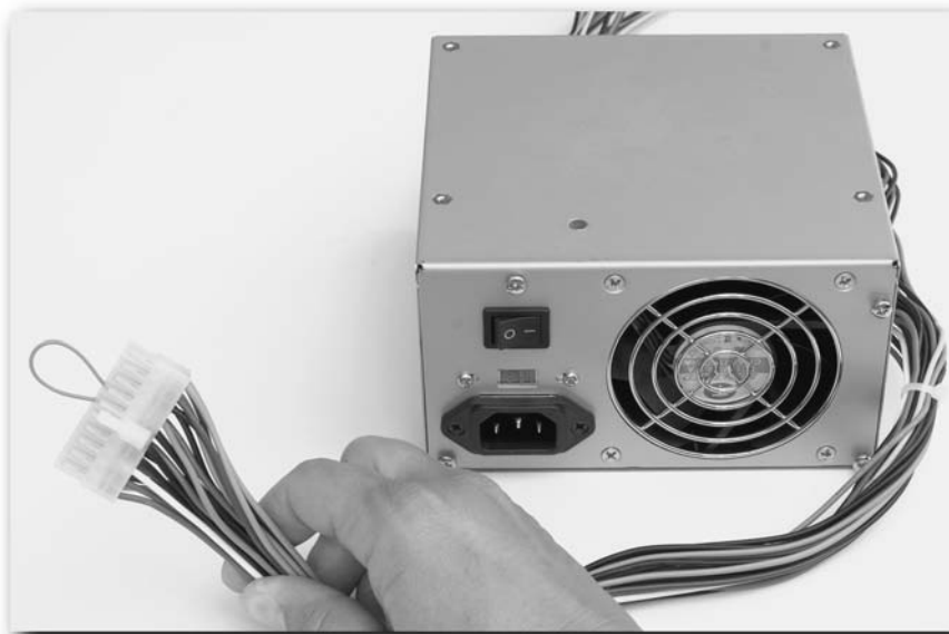
FIGURE 11-16: Jumpering pin 14 to ground.
