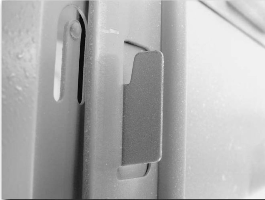
FIGURE 3-5: Metal catches that hold the case together are sturdier than plastic.
