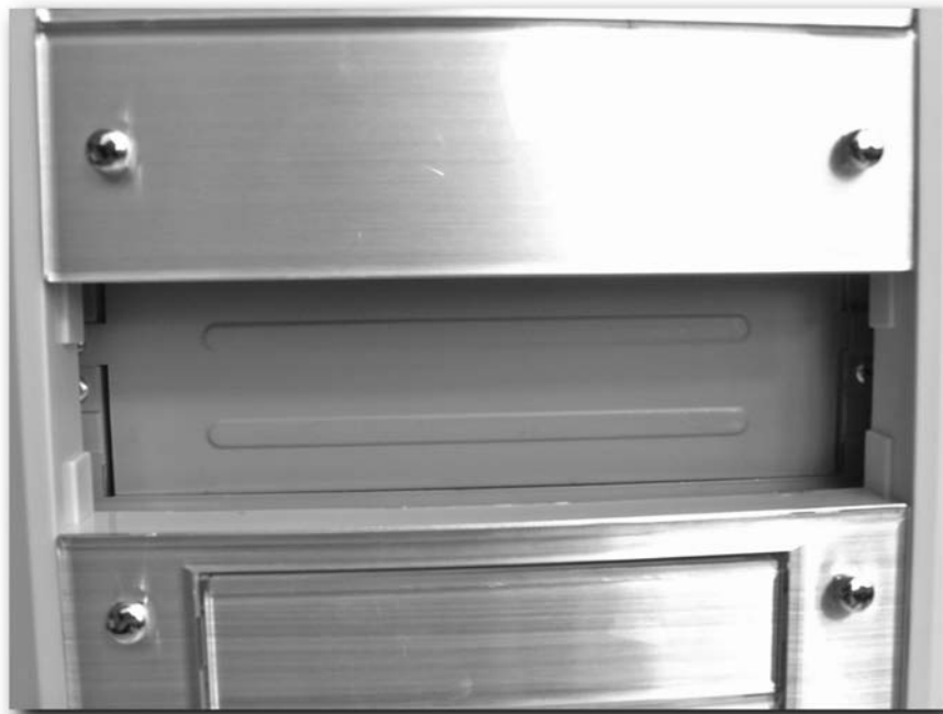
FIGURE 10-27: Metal plate behind fascia.
