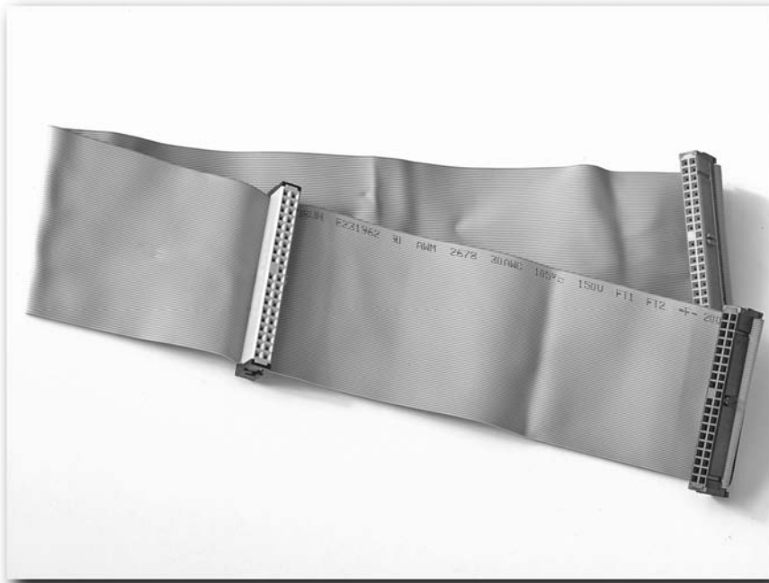
FIGURE 6-6: An 80-wire, 40-pin ribbon data cable.
