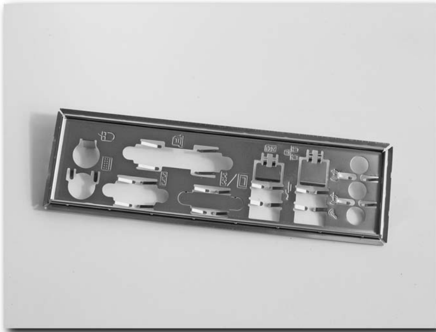
FIGURE 10-28: Motherboard specific connector bezel.
