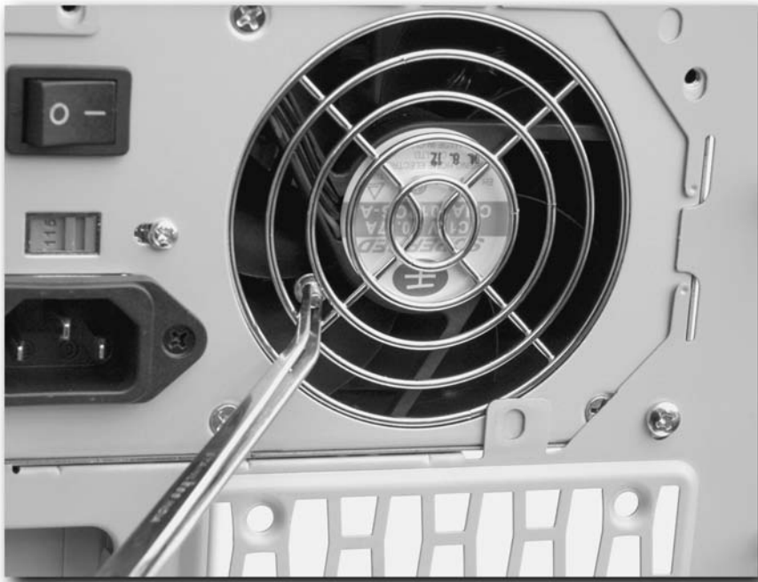
FIGURE 13-7: Screws CAN drop into the PSU!
