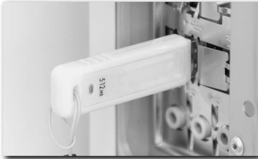
FIGURE 18-4: Checking USB ports with a USB flash memory device.
