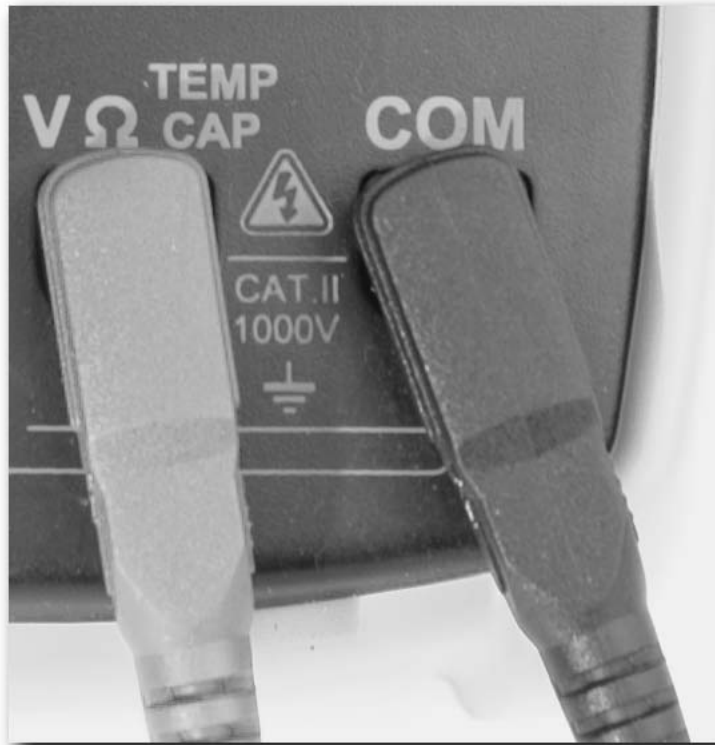
FIGURE 11-17: Probes connected to multimeter.
