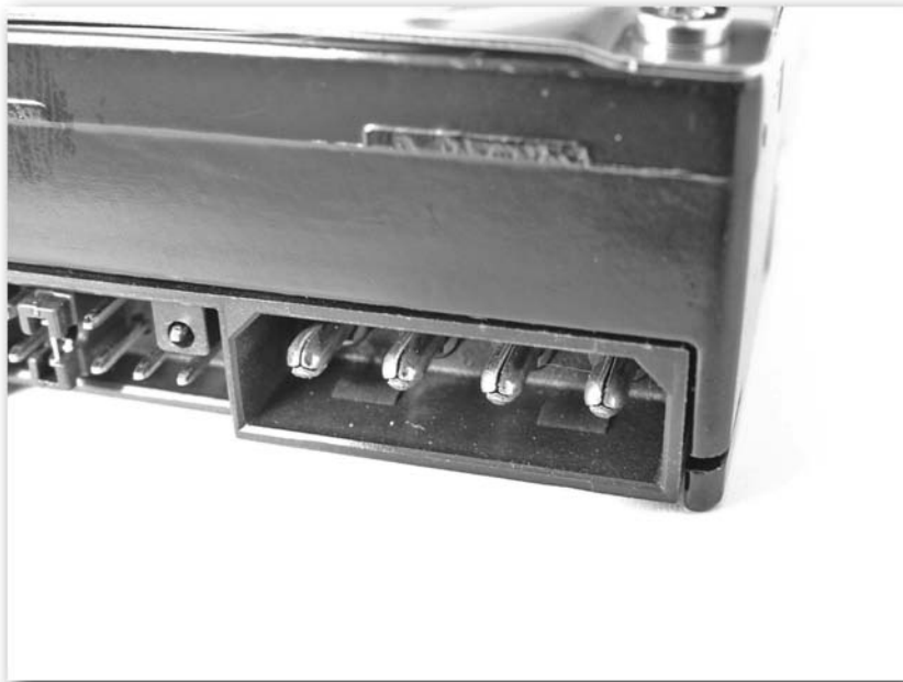
FIGURE 6-4: Power connectors have 4 pins.
