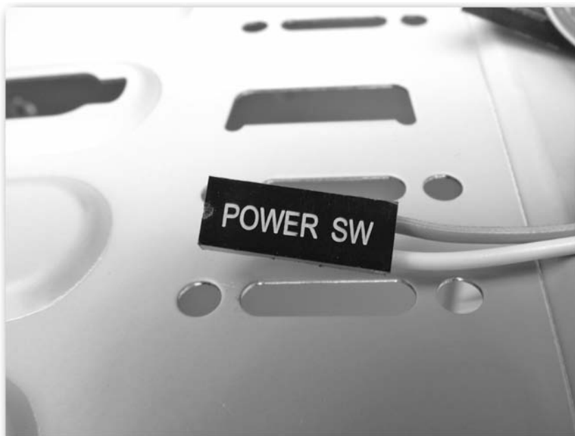
FIGURE 10-7: Power switch lead.
