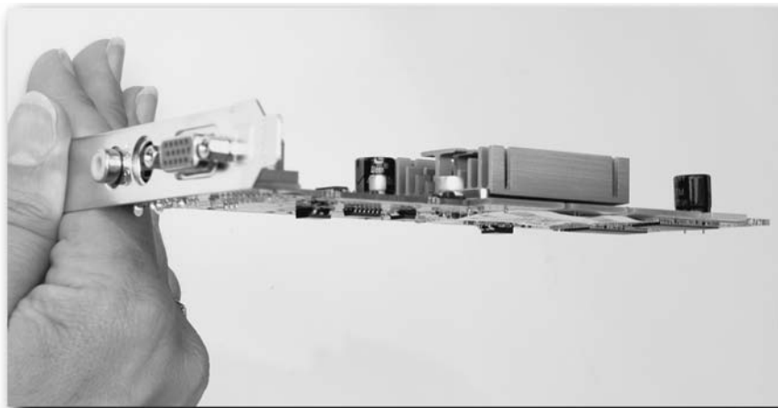
FIGURE 11-1: Carrying out a visual check for warped circuit board.
