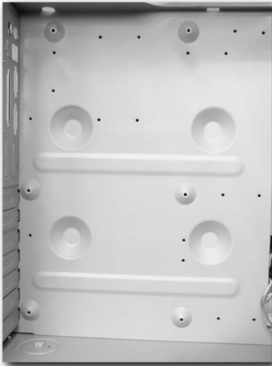
FIGURE 3-2: Screw threads hold the motherboard in place. This shows the relationship between the case and the motherboard.
