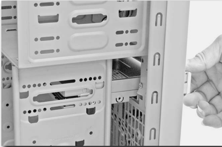
FIGURE 15-3: Fitting the floppy drive.
