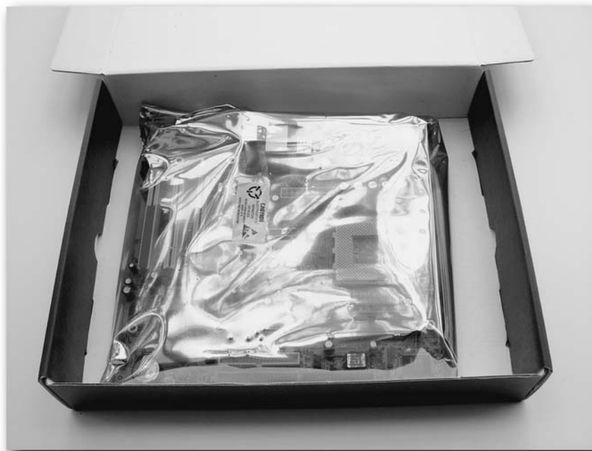
FIGURE 4-7: Safely store your motherboard in an ESD bag until you're ready to use it.
