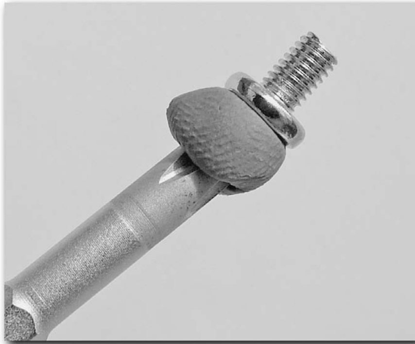
FIGURE 15-5: Improved “magnetic” screwdriver.
