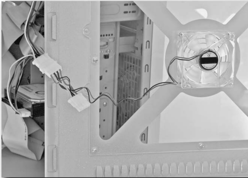
FIGURE 18-3: Connecting up additional case fans.
