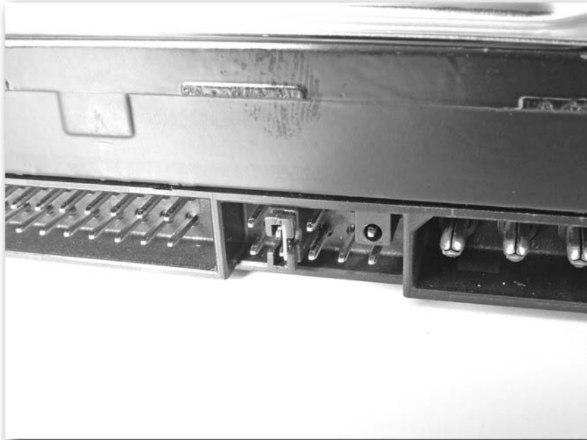
FIGURE 6-5: Drive jumpers allow you to set the primary or secondary drive for the data cable.
