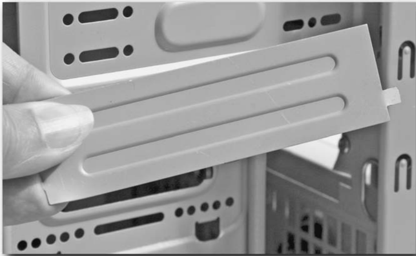
FIGURE 15-2: Metal plate removed from behind fascia.
