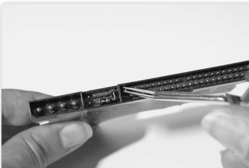
FIGURE 11-11: Using tweezers to straighten the pin.
