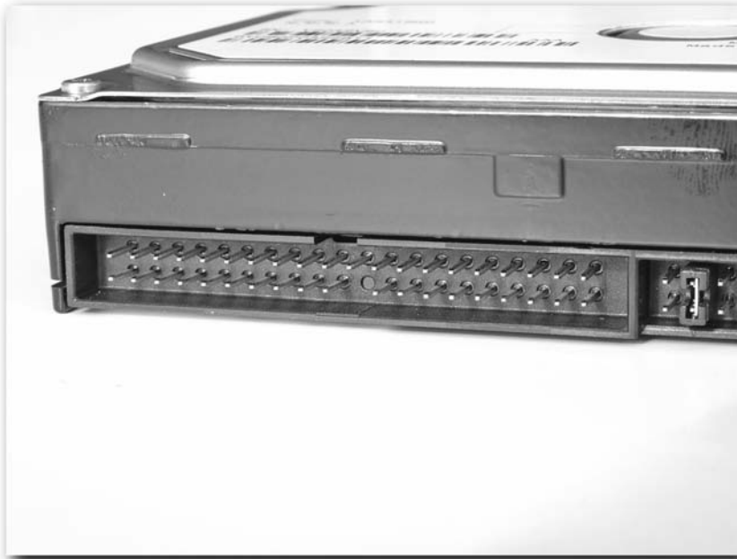
FIGURE 6-3: Data connectors have 39 pins.
