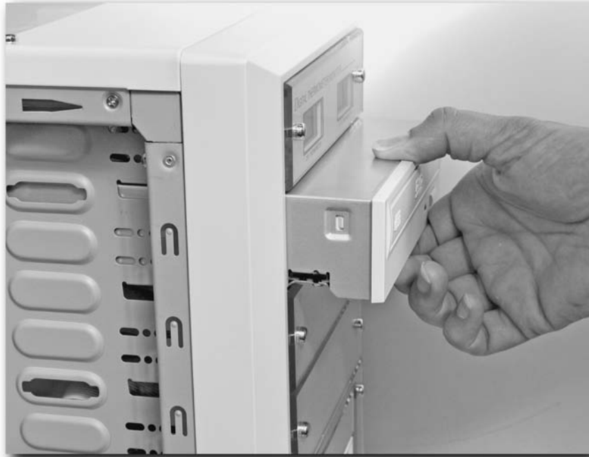
FIGURE 15-14: Fitting the drive.
