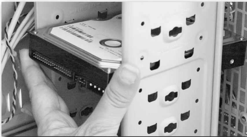
FIGURE 15-9: Fitting the drive.
