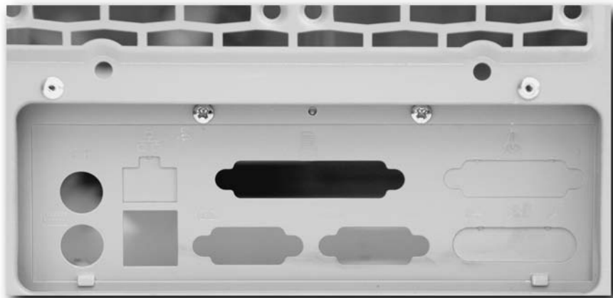
FIGURE 14-6: Generic connector plate on PC case. Note the screws holding the plate in place.
