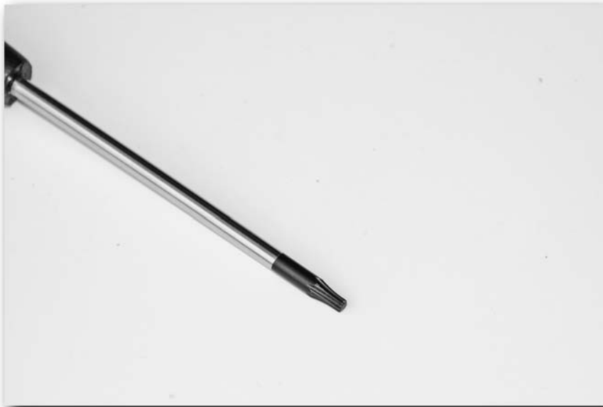
FIGURE 2-3: TORX drivers are rarely used when building PCs.
