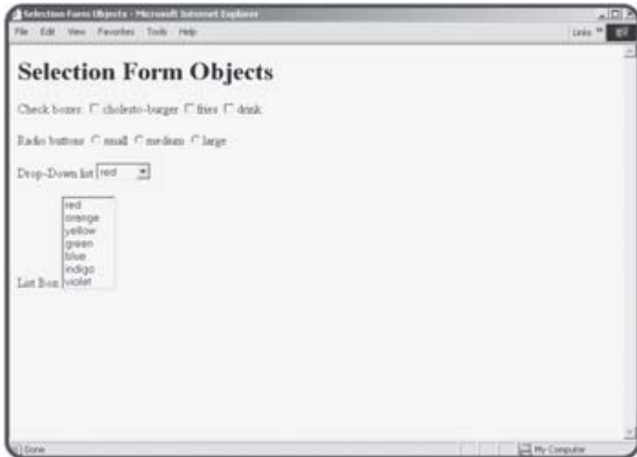
Figure 1.10: Several HTML elements allow the user to enter information without having to type anything.
