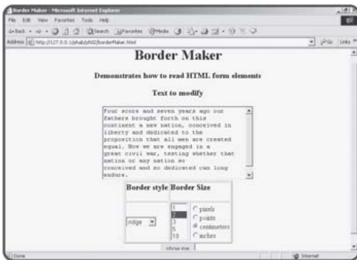
Figure 2.13: The borderMaker HTML page uses a text area, two list boxes, and a select group.
