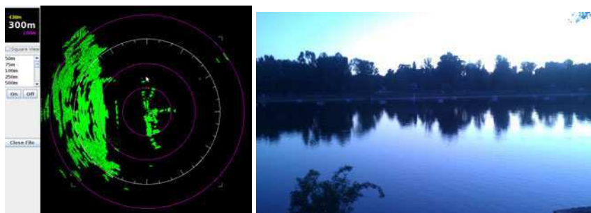
Fig. 7 Radar data/photo comparison "Alte Donau" with buoys (radar port side)
