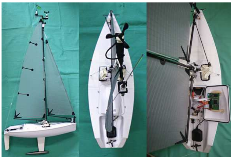
Fig. 1 The figure shows a lateral and top view (left and center) of one of our boats. On the right hand side, a more detailed view of the deck layout and the electronics is shown. In contrast to the conventional design we have mounted the servos on deck and our control board to the lid. Both servos are sealed and a carbon fiber rod is used to connect them to the boom fittings. The black box inside the hull houses the GPS unit, while the black part in the cockpit is the GPS antenna.
