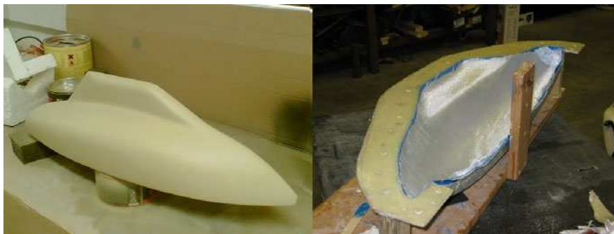
Fig. 4 The plug (left) and the mold (right) for the MOOP hulls
