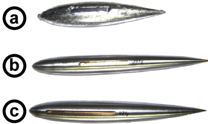
Fig. 3 Three different keel bulbs: a) the standard 370 g bulb, b) a 370 g performance bulb, and c) a 470 g performance bulb
