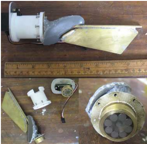
Fig. 5 The rudder assembly, magnetic linkage and servo
