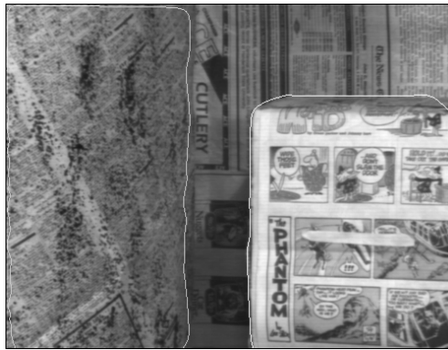
Fig. 8.7. Segmentation of the Cylinder sequence by \mathcal{E}_2 into three regions: The box is distinguished from the background on the basis of optical flow.
