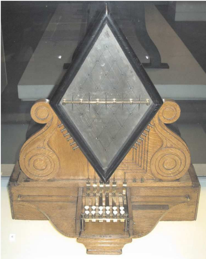
The Cooke and Wheatstone telegraph. The arrangement within the diamond-shaped part of the apparatus is illustrated in Figure 3 .
