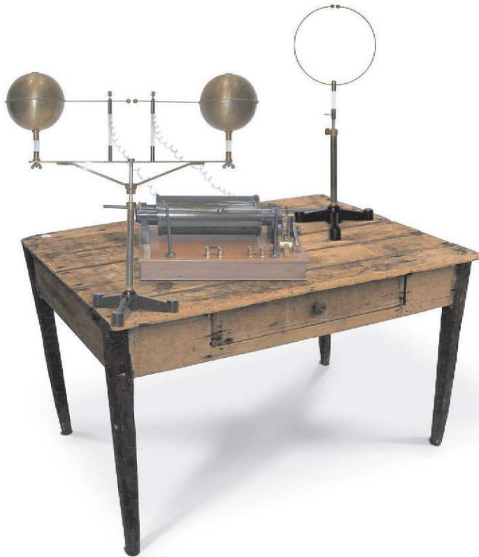
Recreation of Hertz's classic experiment. The transmitter is shown on the left, with the receiver on the right. The induction coil that drives the transmitter is in the center.
