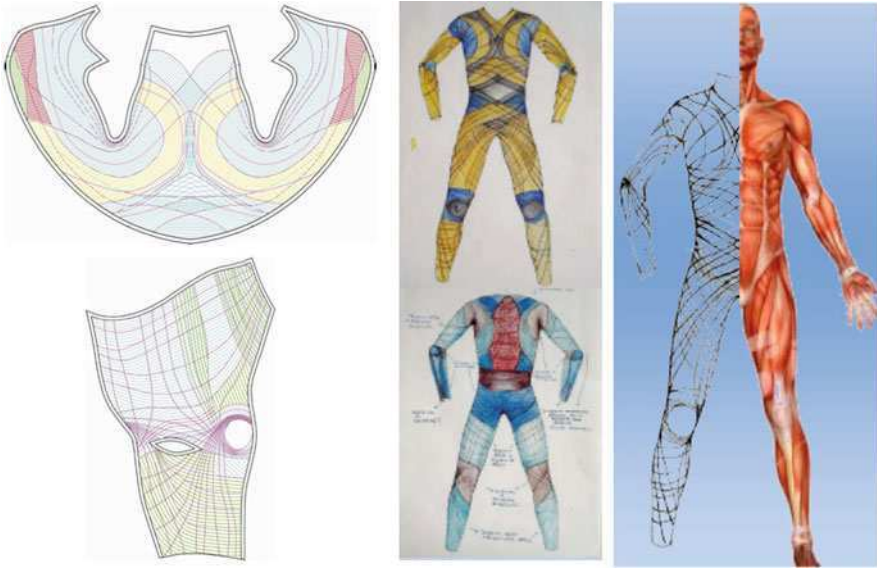
Fig. 11.8 An implementation of second skin lines of nonextension (LoNE) advanced spacesuit design. Thorax pattern ( top left ), thigh pattern ( bottom left ) (credit: Dainese), BioSuit™ concept, LoNE superimposed on musculature
