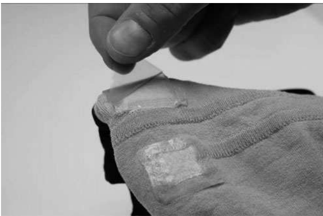
Fig. 7.2 Hydrogel membrane coupled with textile electrode
