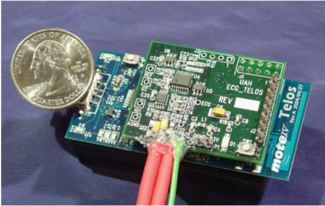
Fig. 3.2 ActiS activity sensor, which incorporates an acceleration/ECG daughtercard interfaced to a Moteiv Telos wireless mote. Courtesy Dr. Emil Jovanov, University of Alabama at Huntsville, USA. Originally published in (Jovanov et al. 2005)
