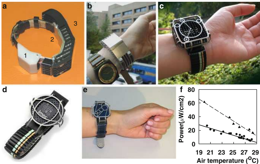
Fig. 2.8 (a) The first wrist TEG: (1) is the electronics module, (2) is a hot plate, and (3) is a radiator. (b) A similar TEG worn next to a watch. (c) A TEG with a pin-featured radiator. (d) A waterproof TEG for outdoor use. (e) A TEG in the wireless sensor for measuring the power generated by people in real life. (f) The power produced by the device shown in (c) in the office on a sitting (circles) and walking (triangles) person
