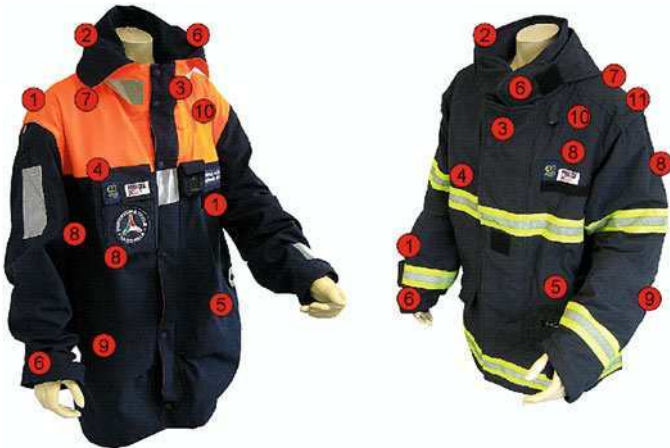
1-Visual alarm module (1x in the FF OG, 2x in the CP OG); 2-acoustic alarm module; 3-external temperature sensor; 4-Wi-Fi communication module; 5-Professional Electronic Box (PEB); 6-triaxial accelerometers (2x); 7-GPS module; 8-Flexible antenna (2x); 9-Flexible battery; 10-CO sensor; 11-Heat flux sensor (only FF OG)
