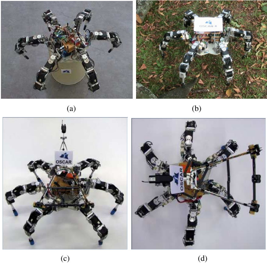
Fig. 3.9 (a) Hexapod robot OSCAR-X in development stage; (b) OSCAR-X in nature; (c) Front view of robot OSCAR-X with onboard camera and additional ultrasonic sensors; (d) Top view of robot OSCAR-X.
