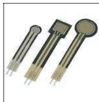
Fig. 3.5 Pressure sensors type FSR-400. The most right one in the figure is used by OSCAR 2.
