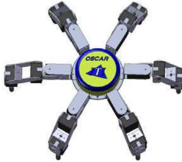
Fig. 3.2 Spatial distribution in circle of legs by OSCAR series of robots.
