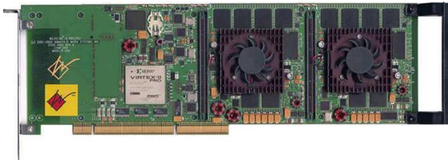
Fig. 1.9 Non real-time compressor based on a COTS board (2 Virtex II Pro FPGA chips on the board)
