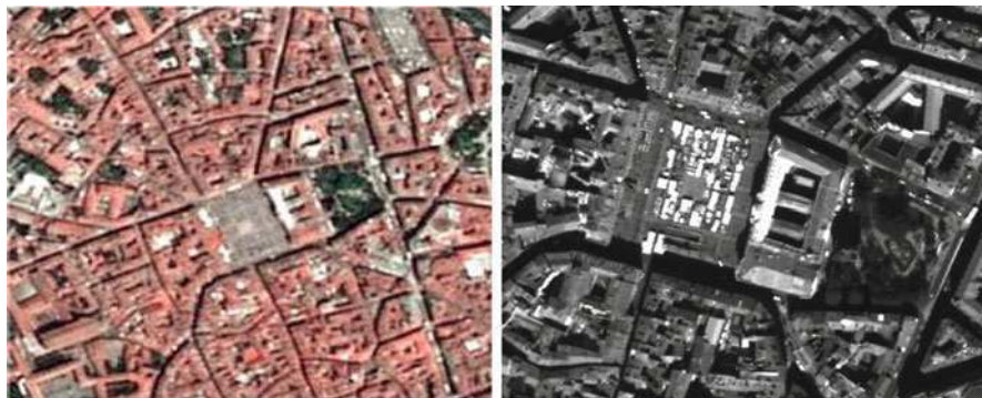
Fig. 2.1 SPOT5 ( left hand side ) and PLEIADES-HR ( right hand side ) images of a famous place in Toulouse. SPOT5 image resolution is 2.5 m and PLEIADES-HR one is 0.7 m
