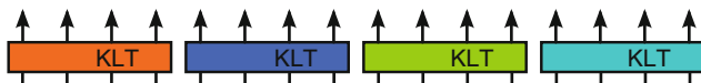
Fig. 10.2 Plain clustering applied to a 16-component image. Each vertical arrow depicts a spectral component as it is transformed by a KLT
