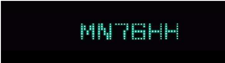
Fig. 3. The displayed image for the fabricated FED panel with CNT field emitters
