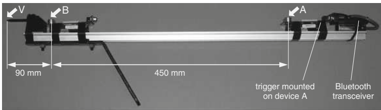
Fig. 3.14 Portable probe prototype of the MScMS-I (Franceschini et al. 2009d). (with permission)
