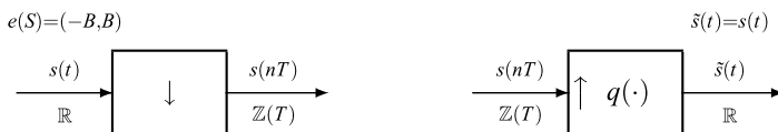
Fig. 8.15 Exact signal recovery from its samples by an interpolator filter under the hypothesis of band limitation and F_c \geq 2B
