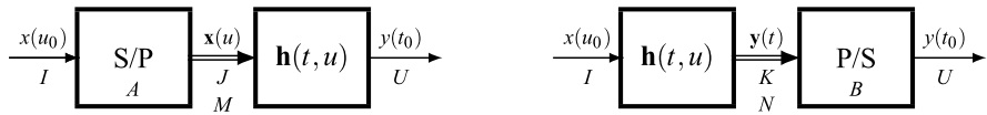
Fig. 7.23 Input decomposition and output decomposition of an I \rightarrow U linear tf
