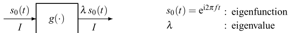
Fig. 5.2 Interpretation of an eigenfunction s_0(t) of a filter: the output signal is proportional to the input signal
