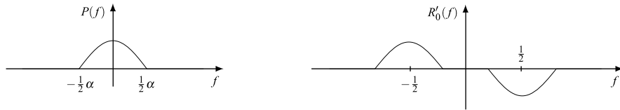
Fig. 9.27 Derivative R'_0(f) of raised cosine for \alpha = 0.6
