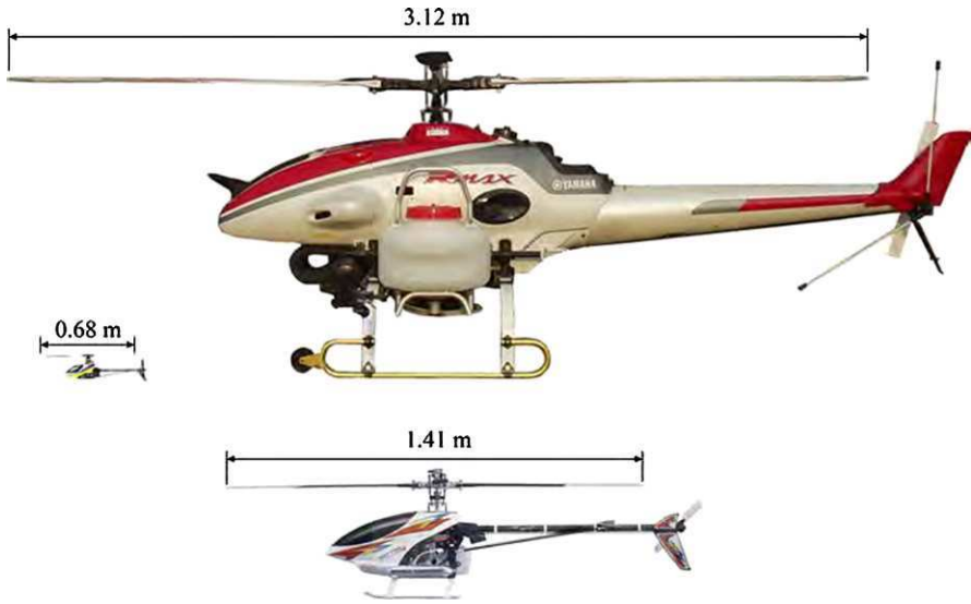
Fig. 1.6 Examples of Type I (Rmax), II (Raptor 90 SE), and III (TREX 450) rotorcraft
