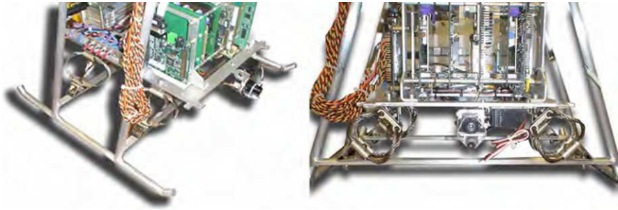
Fig. 3.12 Anti-vibration design for the onboard computer system (left: side view, right: front view)
