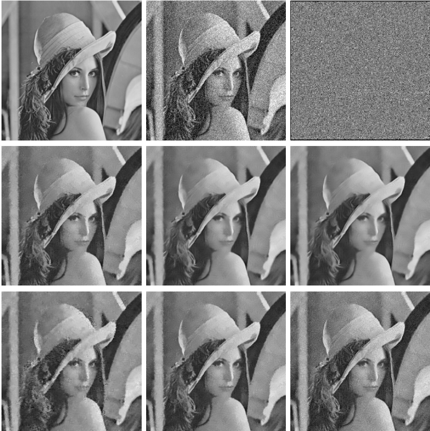
Fig. 2. Kernel functions performance with different images based on NLM method. From left to right, up to bottom are original image, noise image (20.14 dB), denoised by original NLM (25.50 dB), Kaiser Window function NLM (29.31dB), average patch difference (29.11 dB), median patch difference (25.62 dB), Laplacian kernel function (28.53 dB) and Mexican hat wavelet kernel function (25.67 dB), respectively.
