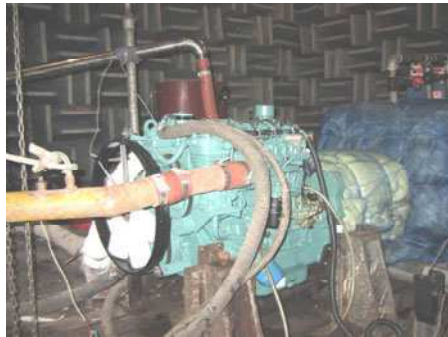
Fig. 1. Diesel engine and dynamometer installation diagram
