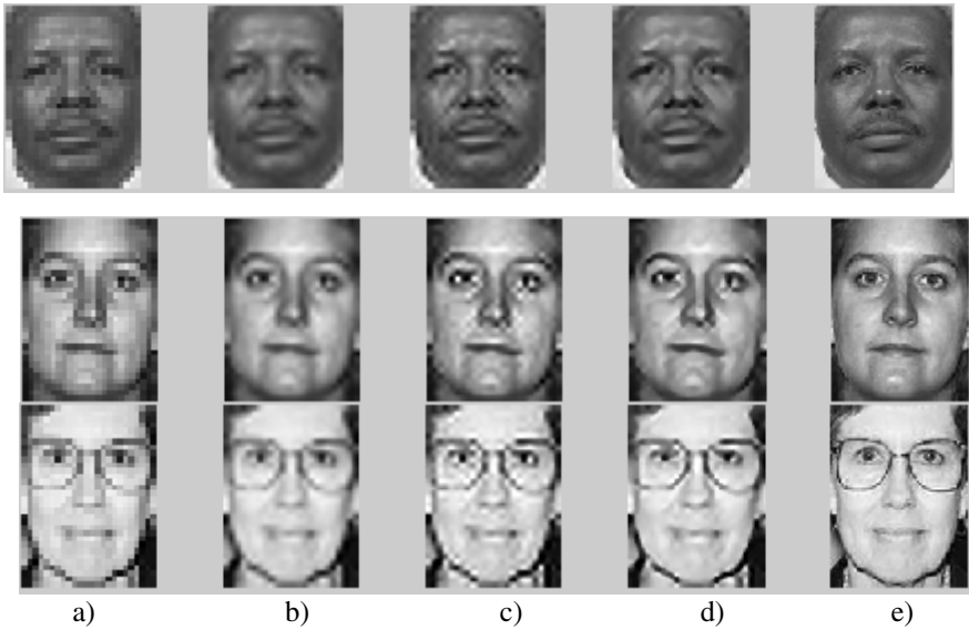
Fig. 1. Visual comparison results ( a)low-resolution b) Bicubic Interpolation c)example-based method d)paper's method e)original image)
