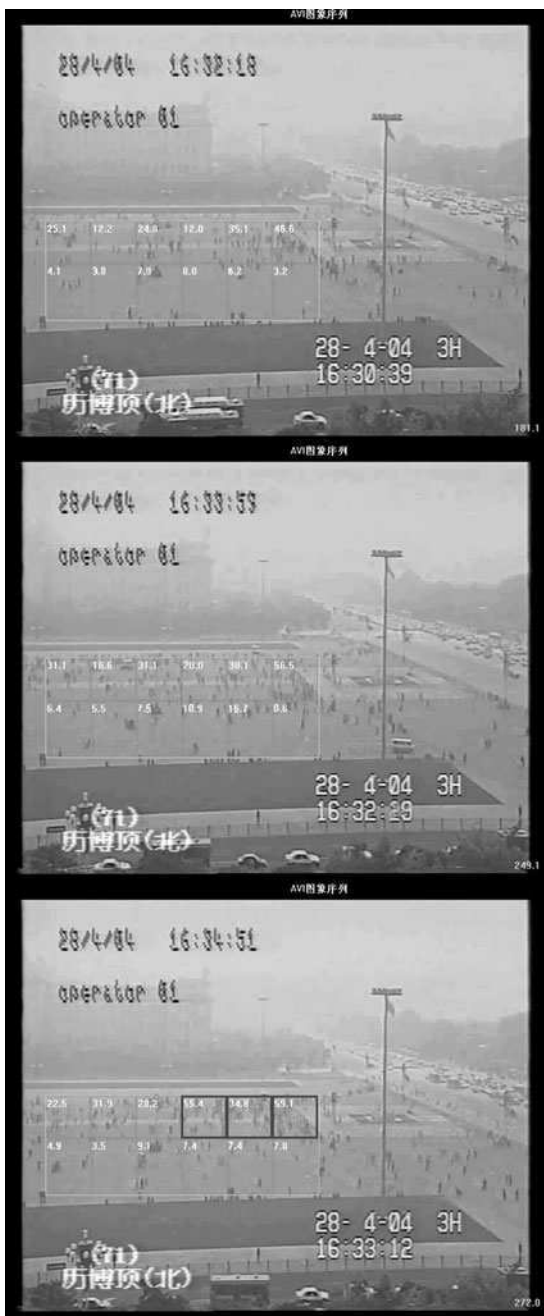
Fig. 7.17 The overcrowded situation detected from a video of Tian'anmen Square (the numbers are the estimated number of people in each cell).
