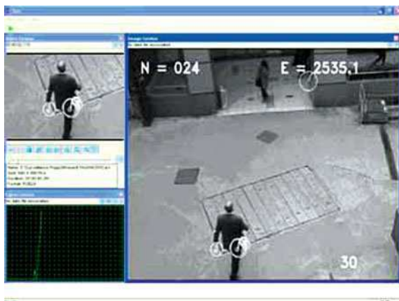
Fig. 8.8 Interface of the metro video surveillance system.
