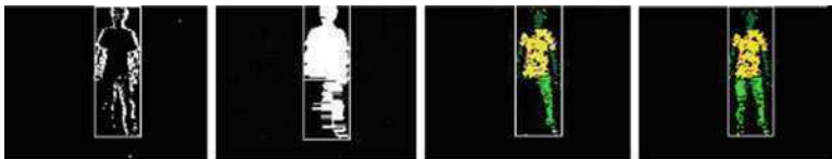
(a) Frame differencing result (b) The blob filling result (c) The middle labeling result (d) The last labeling result
