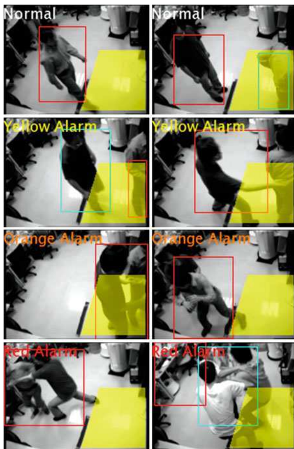
Fig. 8.18 Quad Snapshots of experimental results. The semitransparent yellow region is the sensitive area we defined at beginning. The rectangle on the people means that their motion is being tracked. The Yellow Alarm indicates that someone is striding over the yellow line when a customer is operating on the ATM. The Red Alarm warns of the occurrence of violence. The left sub-figure of Orange alarm indicate more than one customer in the area, and the right sub-figure shows the interim of violence behaviors.
