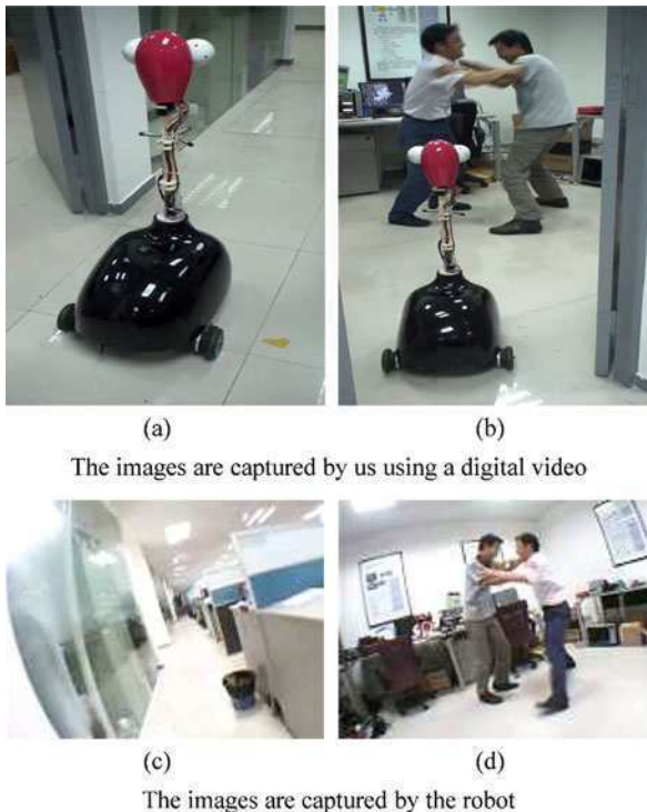
Fig. 4.19 The process of abnormal behavior detection utilizing video and audio information: (a) The initial state of the robot; (b) The robot turns to the direction where abnormality occurs; (c) The initial image captured by the robot; (d) The image captured by the robot after turning to direction of abnormality.
