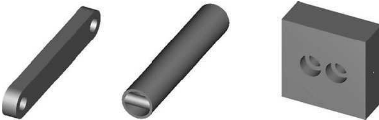
Fig. 10.47 Design features—piston elements and back wall
