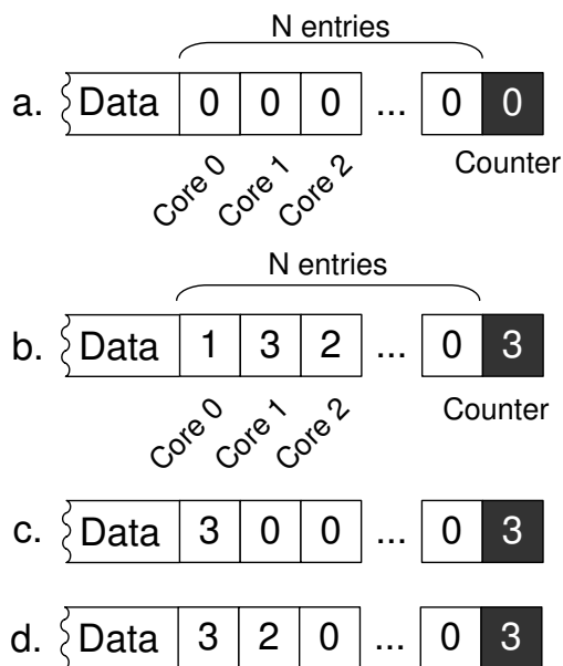
Fig. 5.3 Dacota access vector. An access vector associated with each cache line is used to track the order of store operations. a. Access vector at the beginning of an epoch. b. Access vector indicating modifications (in order) by core 0, core 2 and core 1. c. and d. Examples of aliasing due to multiple store operations by a same core. In c. it can be inferred that core 0 performed three store operations, because the other access vector entries are all 0; in d. the complete order of operations cannot be recovered: either core 0 or core 1 performed the first store operation, but we cannot infer which of the two.
