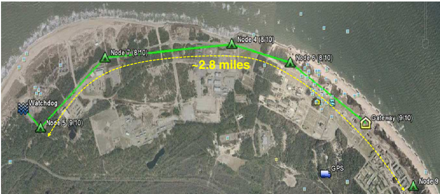
Fig. 21.6 Long-endurance field experiment network topology with power-enhanced CC1110 radio at Norfolk, VA. About 3 miles of shoreline was covered with six (static) Relay-mode nodes to track target objects (either vehicle or a boat). The numbers next to the Node ID (9/10 or 8/10) indicate remaining battery reserves after 3-week experiment, confirming that their power consumption behaviors offer at least 6 months of lifetime with 250kJ batteries.
