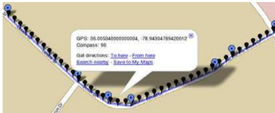
Fig. 10.2 Large blue icons mark the piecewise segments of the polyline, while black icons are computed intermediate points. Each location associated with the latitude, longitude and the angle from magnetic north.
