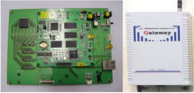
Fig. 4 Green control gateway H/W
