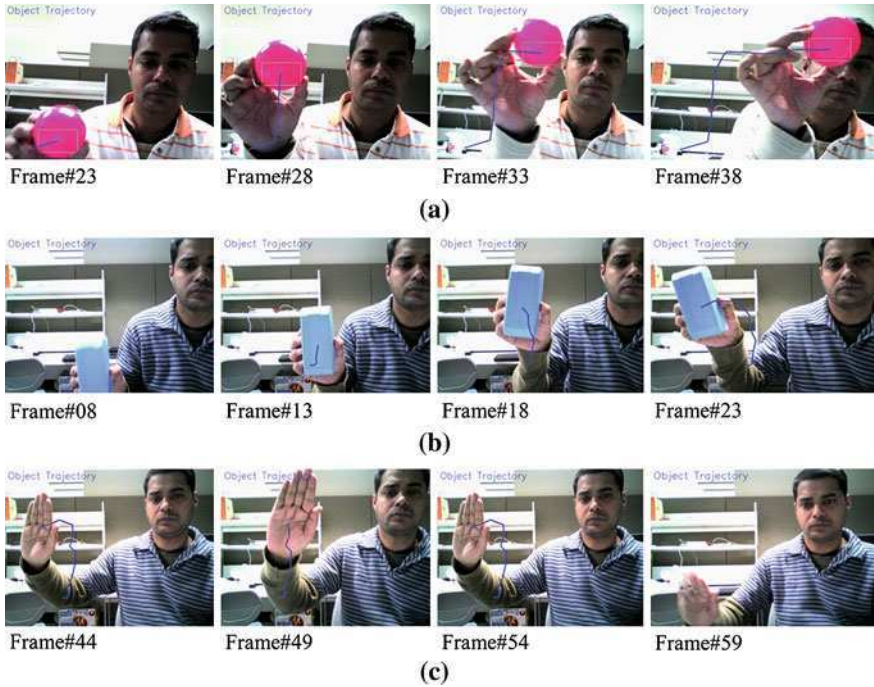
Fig. 2 Example outputs of trajectory generation method. a Trajectory of a “Pink Ball” (clip #1). b Trajectory of a “Duster” (clip #2). c Trajectory of a “Hand Palm” (clip #3)
