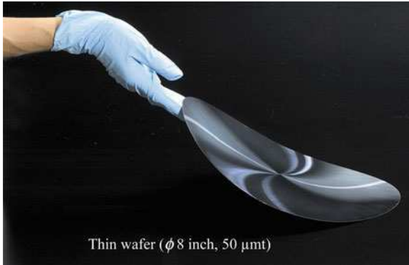
Fig. 5.1 Thinned wafer showing lack of mechanical stiffness
