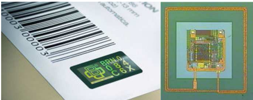
Fig. 31.15 Security tag [6] and UCODE chip with integrated RF antenna
