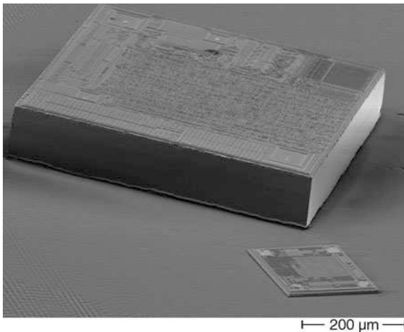
Fig. 4.6 Two RFID chips of a thickness of 260 \mu\text{m} (Philips ICode) and 25 \mu\text{m} (NXP UCode, in front, size 0.4 \times 0.4 mm). The shrinkage in size illustrates the ongoing miniaturisation of microelectronic devices
