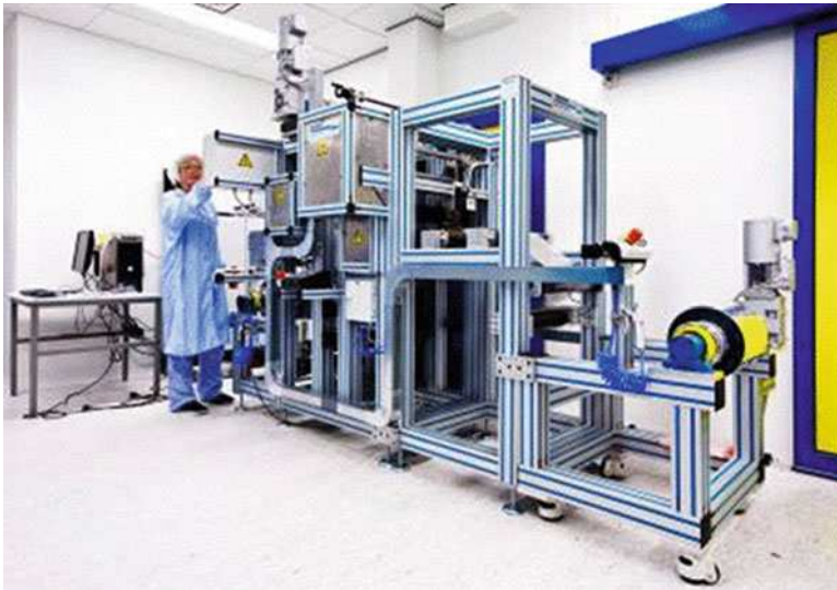
Fig. 13.3 R2R lamination line (at Holst Centre, Eindhoven)
