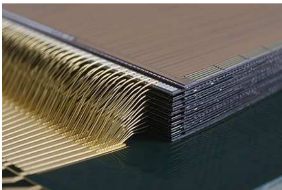
Fig. 15.1 Multi chip package with 20-30- \mu\text{m} -dies (Courtesy of Elpida Memory, Inc. [JP])
