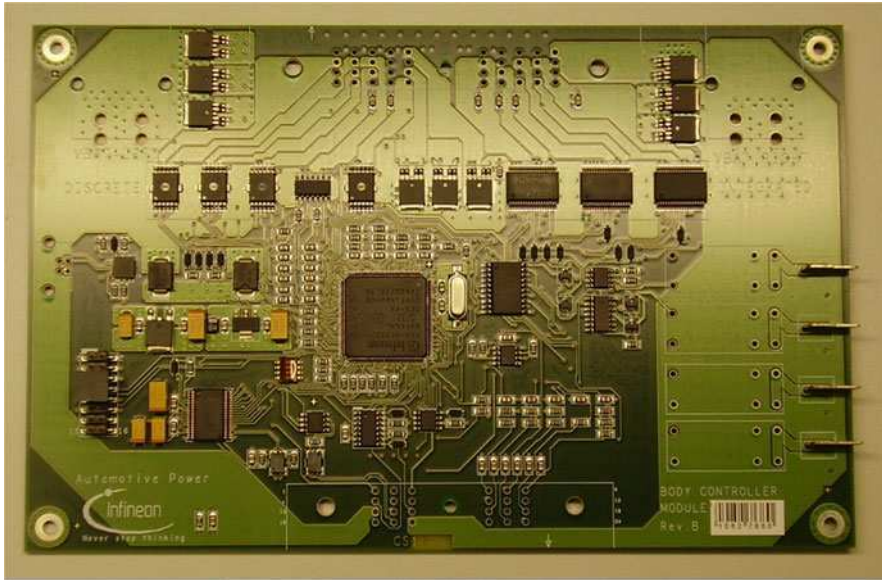
Fig. 25.13 Typical automotive module realized with Infineon semiconductor devices
