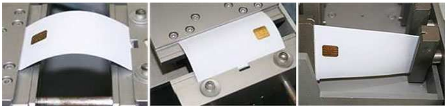
Fig. 31.4 ISO bending and torsion tests
