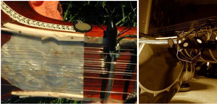
Fig. 13.5 FSR sensor used to measure thumb pressure on ESitar 1.0 (left) and ESitar 2.0 (right).
