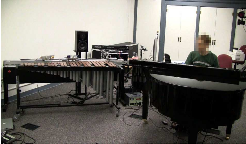
Fig 14.6 Experimental setup showing the human pianist on the right, and the robotic marimba player Shimon on the left.
