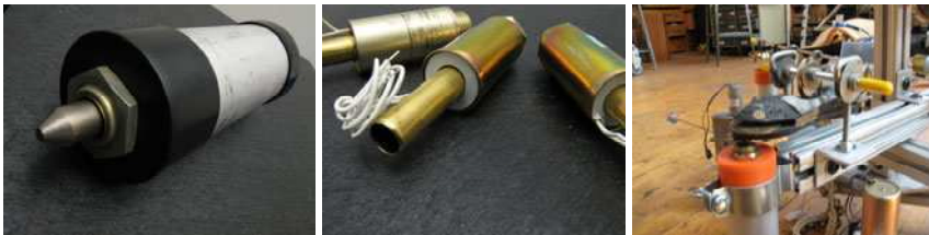
Fig. 13.10 Trimpin BellHop outside shell tubing (left) and inside extended tubing (middle). Trimpin BellHops used on MahaDeviBot (right).
