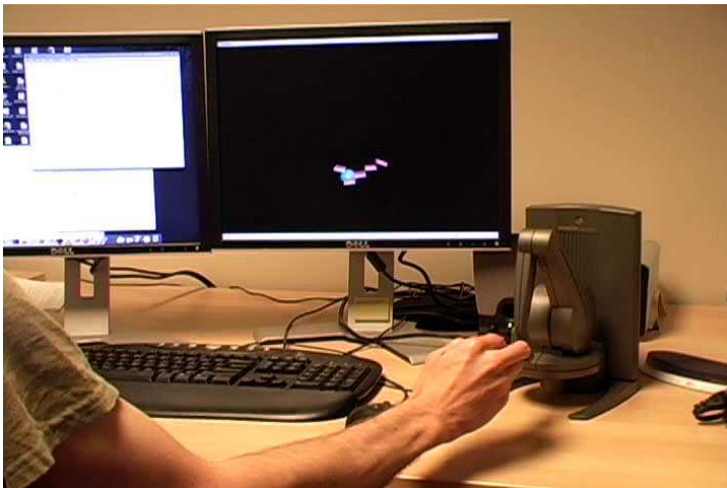
Fig. 5.5 A user interacting through a haptic device with a set of mutually constrained shapes in DIMPLE. Each object controls a frequency modulation synthesizer. The user is manipulating a Phantom Desktop haptic device from SensAble Technologies.
