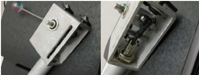
Fig. 13.8 Singer Hammer with added ball-joint striking mechanism.
