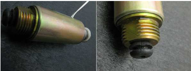
Fig. 13.7 Kapur Finger using a grommet and padding.
