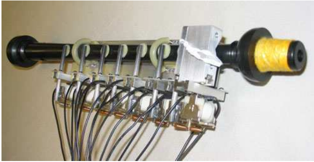
Fig. 10.4 Chanter is mounted on aluminum block along with electromagnetic coils that open and close sound holes using rubber pads at the end of lightweight plastic tubes.
