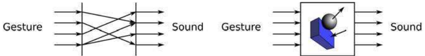
Fig. 5.4 Abstract functional gesture-sound mapping (left) vs. mapping based on a virtual instrument layer (right).
