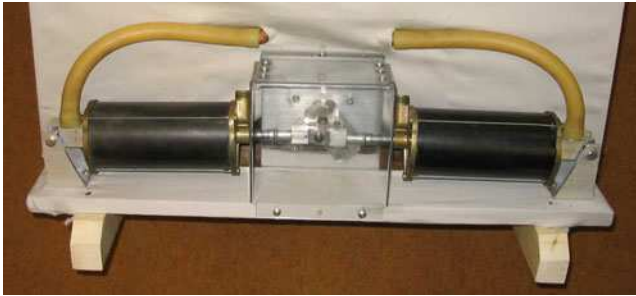
Fig. 10.3 The McBlare air compressor. Electric motor (not visible) drives eccentric (center) through a gearbox. Eccentric drives two air pump cylinders (right and left) in opposition.
