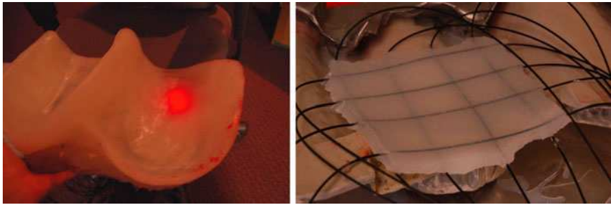
Fig. 5.3 Initial interface prototype for the Ballagumi (left), showing optical sensor grid (right).
