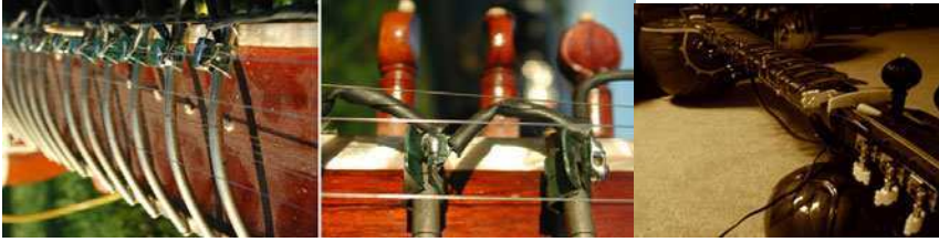
Fig. 13.4 The network of resistors on the frets of the ESitar 1.0 (left, middle). The ESitar 2.0 full body view (right).
