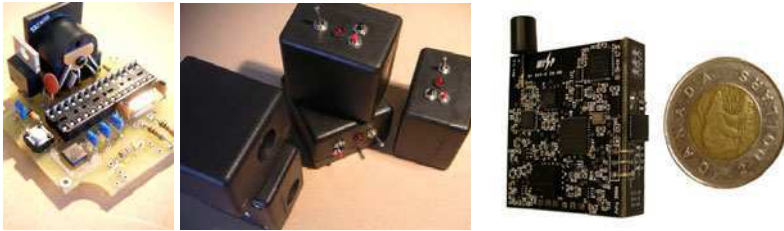
Fig. 13.6 The KiOm Circuit Boards and Encasement (left, middle). Wireless Inertial Sensor Package ( WISP ) (right).
