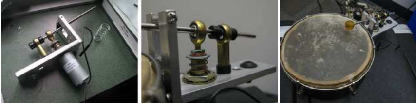
Fig. 13.9 Trimpin Hammer modified to fit the MahaDeviBot schematic.
