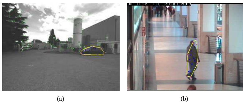
Fig. 5. Object contour initialization, for a rigid moving object, image (a), and non-rigid moving object, image (b)
