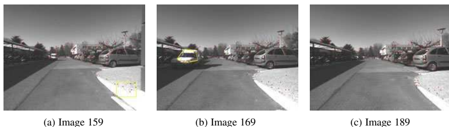
Fig. 10. Outdoor experimental results at higher velocity. Two dynamic objects are detected: a false moving object on the ground and a real moving truck (see the text for a more detailed explanation).
