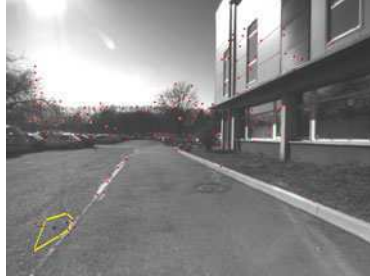
Fig. 3. False dynamic object detected on the ground for higher motion velocity
