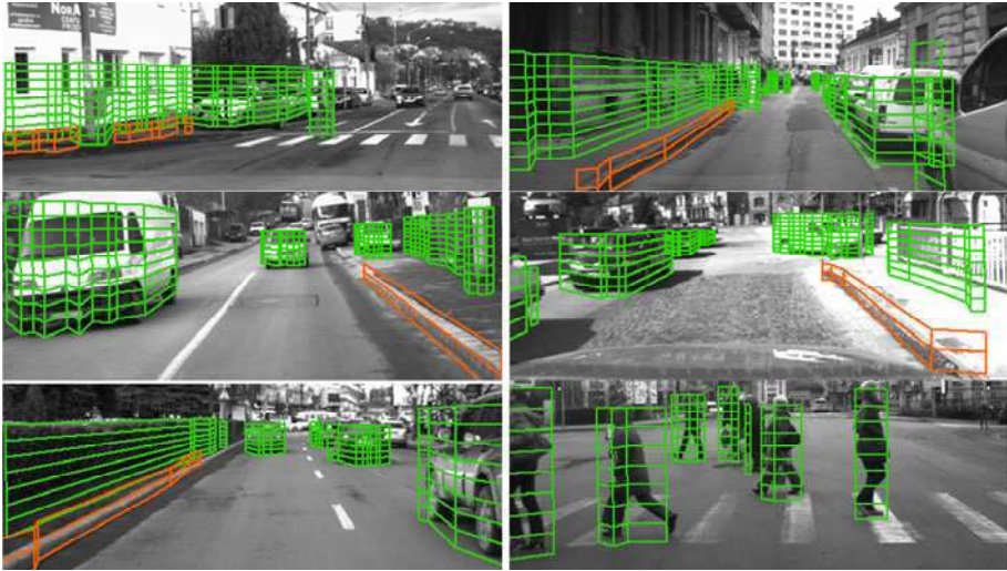
Fig. 11. Object delimiters detection through the Combined Border Scanning algorithm for various traffic scenes. The delimiters are projected onto the Left Image and are represented as grids labeled as Traffic Isles (orange) or Objects (light green). The grid height is the same as the enveloped object by the current delimiter.
