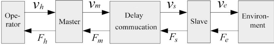
Fig. 1. Basic Bilateral Teleoperation Scheme
