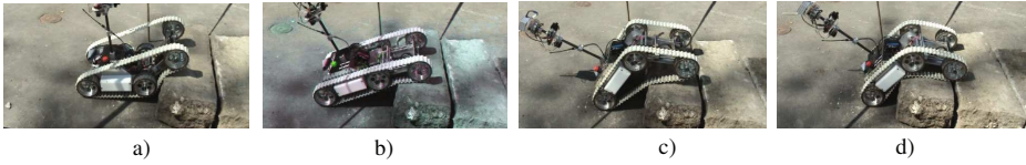
Fig. 3. B2P2: Clearing of a curb
