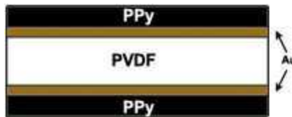
Fig. 4. General structure of trilayer polymer actuator
