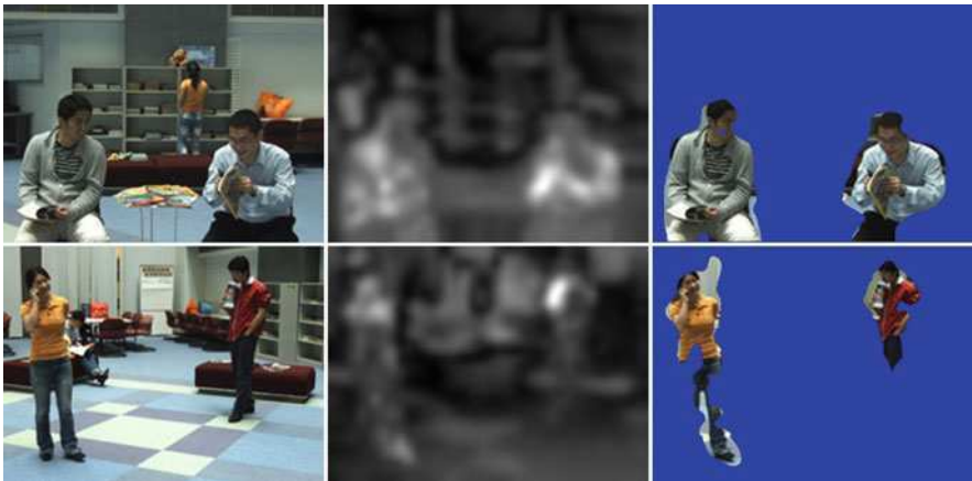
Fig. 5.3 Automatic object extraction: left : input image; middle : saliency map; right : initial OOIs; top : Reading sequence; bottom : Calling sequence
