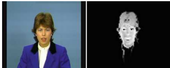
Fig. 1.9 An example of facial saliency map. Left: Original image claire . Right: The facial saliency map
