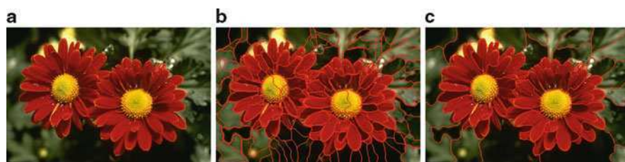
Fig. 1.5 An example of superpixel segmentation. (a) Original image flower . (b) Superpixel map with the number of 200. (c) Segmentation result based on the superpixel map
