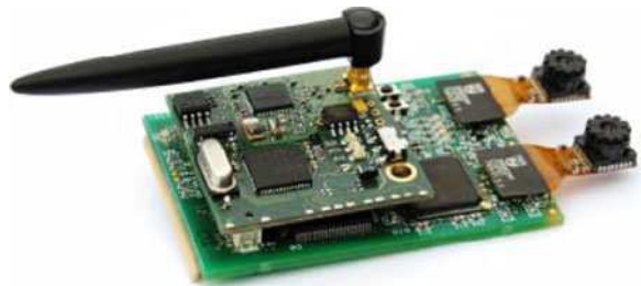
Fig. 4.14 NXP Semiconductors' WiCa wireless smart camera board
