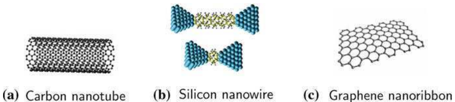
Fig. 1.9 Low dimensional structures as channel replacement: a CNTs are rolled graphene sheets. b SiNWs are Si atoms in a bulk arrangement, having variable length and cross-section dimensions (shown here with contacts). c Graphene nanoribbons are narrow graphene stripes
