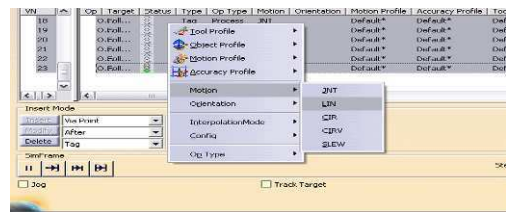
Fig. 40 Screenshots for selection of all tags in linear motion for predefined activity.
