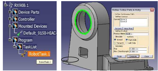
Fig. 20 Snapshots windows for the selection of follow path activity under robot task
