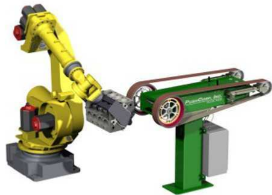
Fig. 10 Illustration of force/torque sensor in grinding process
