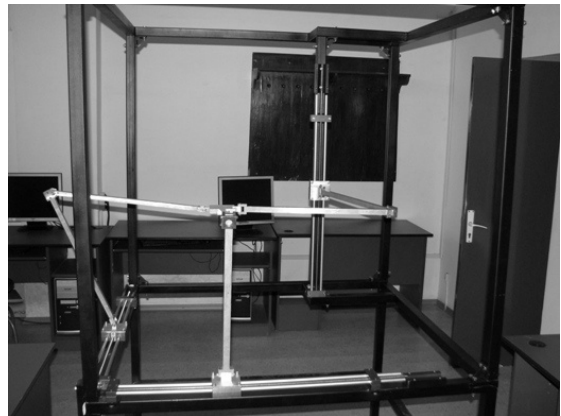
Fig. 1. 3 DOF Isoglide3 parallel robot.
