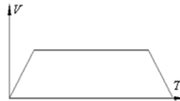
Fig. 2 Multi Segment Feedrate Profile with Feedrate Smoothing Treatment
