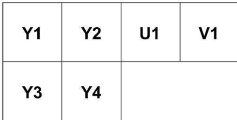
Fig. 1. YUV 4:2:2 pixel format and single video frame storage.
